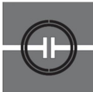
Figure 34 A unit cell of CRLH transmission line. Figure extracted and edited from [19].
