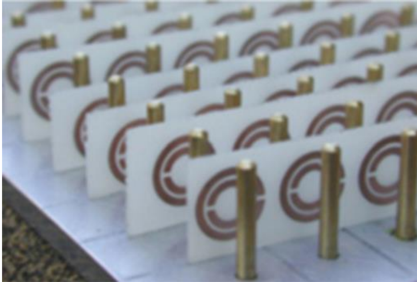
Figure 14 Effective left-handed artificial media (LHM) formed by a combination of ENG and MNG medias. Figure extracted and edited from [3].
