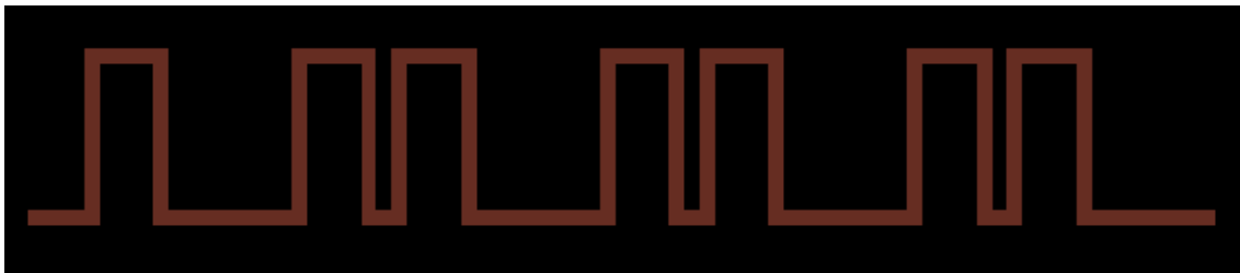
Figure 4.19: Layout of the artificial transmission line of the second stub implemented with N = 4
