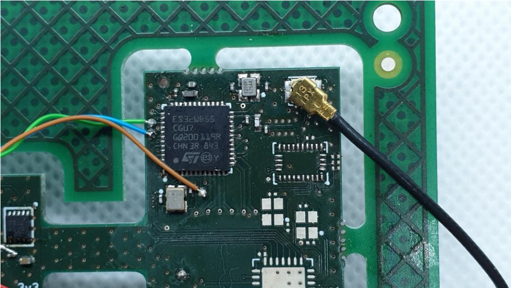
Figure 40 Close Up of the MCU and other components.
