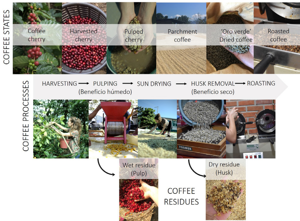
Figure 5.6: Timeline describing coffee evolution from coffee cherry state to roasted coffee and the associated processes and residues. Described the wet processing methodology. All photographs were taken during the visits to coffee growing communities in Chiapas, Mexico.
