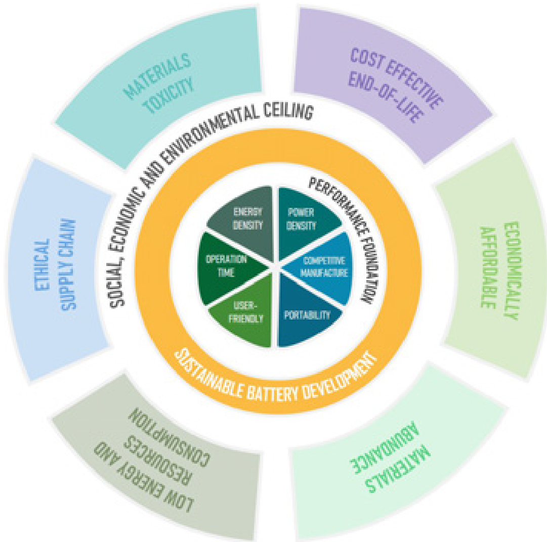
Figure 2.2: Defining a sustainable space for batteries development. The six dimensions that define the performance foundation ensure the power supply for the portable battery application. The six dimensions of the social, economic and environmental ceiling prevent the battery to exceed the natural planetary boundaries and ensure a just and accessible technology.
