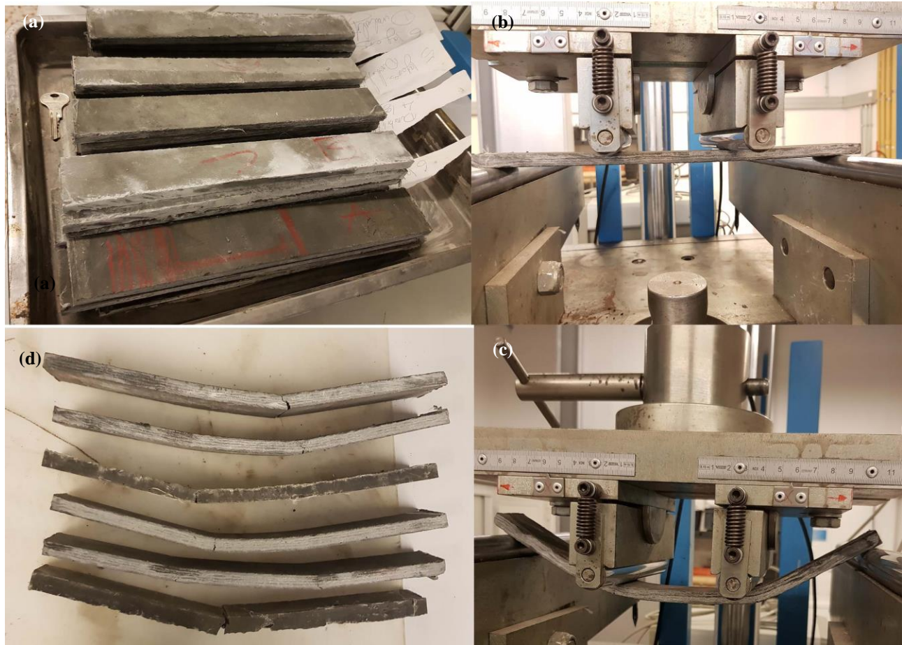
Figure 6. Flexural tests set-up: (a) specimens; (b) flexural test configuration-initial of the test; (c) flexural test configuration-end of the test; (d) Cross-sections of tested-to-failure specimens
