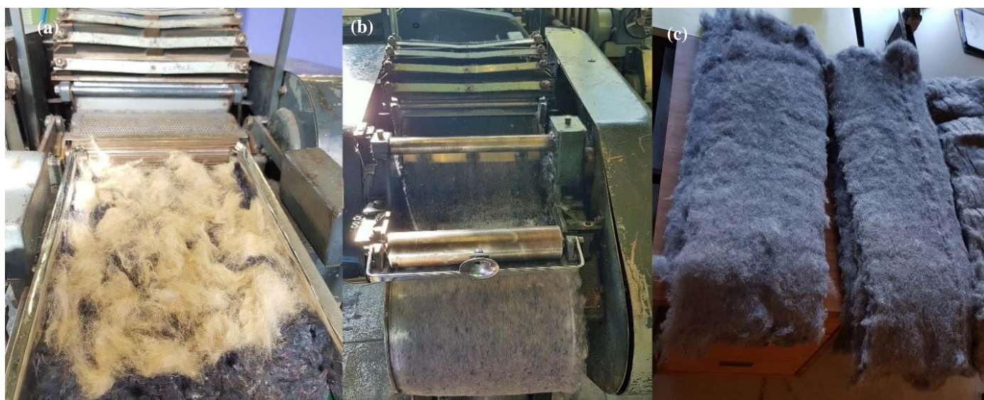
Figure 2. Carding process: (a) opening the fibers in 3 layers; (b) carding; (c) final batts
