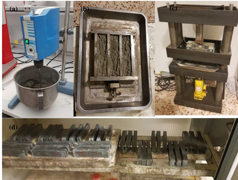
Figure 2. Preparation of the samples: (a) mixing process; (b) molds filled with material; (c) compression and water excess elimination process and (d) curing conditions
