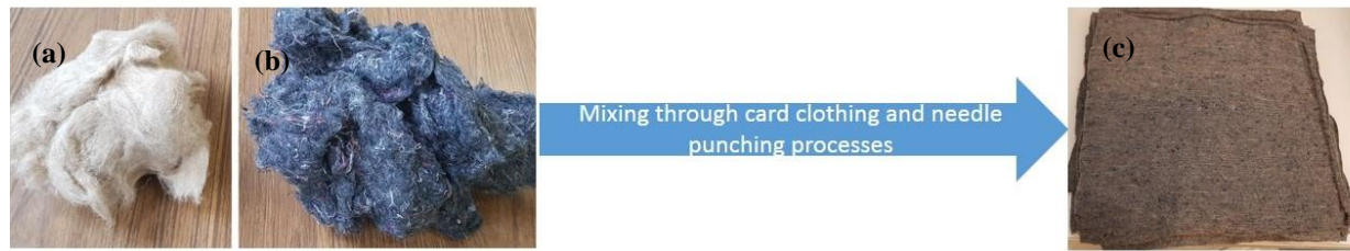
Figure 1. (a) flax fiber; (b) textile waste fiber; (c) final nonwoven fabric.
