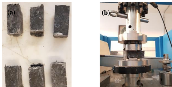
Figure 4. Compressive strength tests: (a) remaining halves of the flexural tests and (b) test configuration
