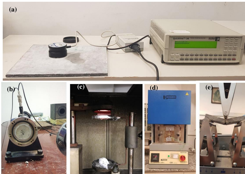
Figure 2 . Experimental setup: a) thermal test; b) acoustic test; c) epiradiator test; d) oven for small-scale fire resistance test ; e) three-point flexural tests setup
