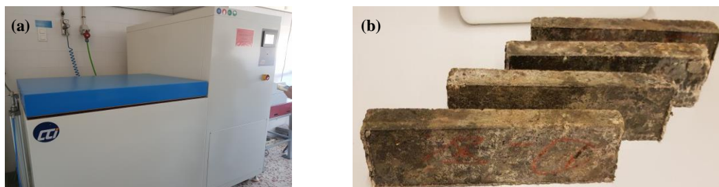
Figure 5. Durability test: (a) CCI chamber (b) Specimens after 25 cycles
