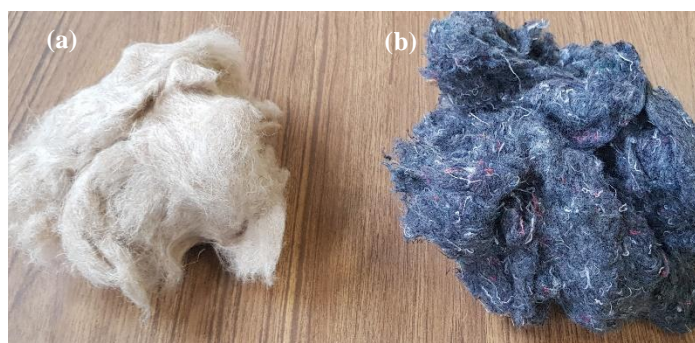
Figure 1. (a) Long Flax Fiber (F); (b) Short Textile Waste Fiber (TW)
