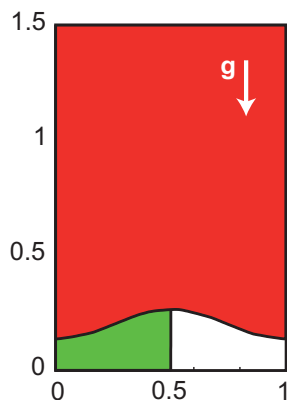
Figure 4.10 – Initial configuration composed of three materials. The upper material is denser than the other two. The viscosity of the materials for each particular simulation is indicated on the caption of Figure 4.12.
