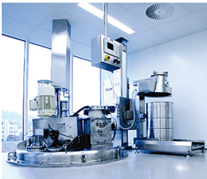
Fig. 3. Milling and mixing centre. Automated and closed drum infeed system in the new milling and mixing centre.
