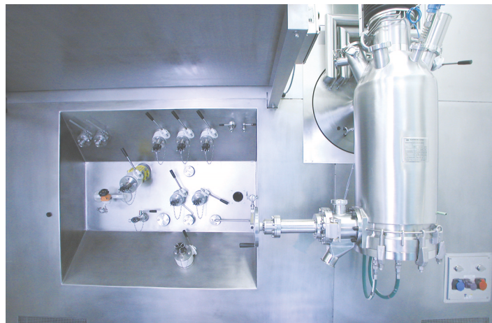
Fig. 4. Filter dryer in pilot laboratory. The filter dryer is located immediately next to the crystalliser. This ideal solution allows product losses during isolation to be kept to a minimum. The closed system prevents product contamination and makes the plants easier to operate and to clean. The systematic separation of workroom and technical installations is totally new in the area of small-volume production. This separation simplifies the cleaning operations, which are confined only to the workroom and the reactor room. This allows rapid product change.
