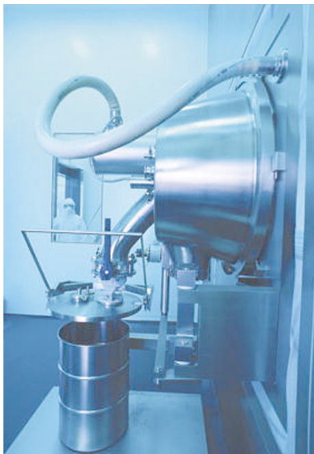
Fig. 6. Centrifuges and drying room. In the pilot, two automatic horizontal centrifuges and a ball dryer are installed. The centrifuges are made of chemically resistant Hastelloy C22 and are therefore also suitable for handling hydrochlorides. All installations are computer-controlled. The workrooms contain only a minimum of technical installations. All surfaces are chemically resistant.
