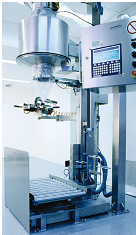
Fig. 5. Milling and mixing centre. Automated and closed filling station in the new milling and mixing centre.
