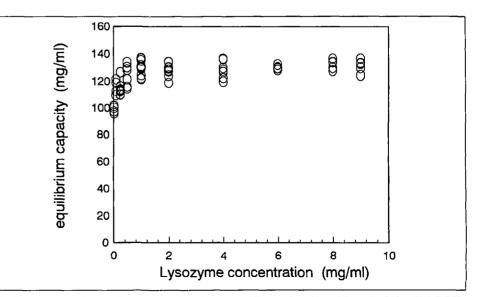
Fig. 2. Binding isotherm of lysozyme to Sartobind S membrane absorbent (25 mM AcONa, pH 4.5, 25°)
