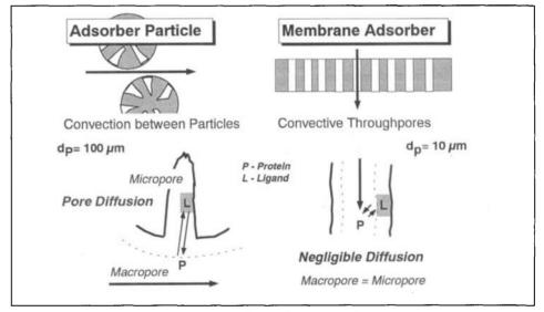
Fig. 1. Comparing membrane- and particle-based chromatography
