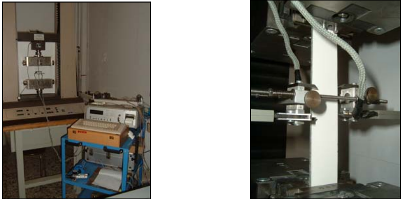
Fig. 6 - Housfield, UPM 100, and specimen equipped by extensometer
