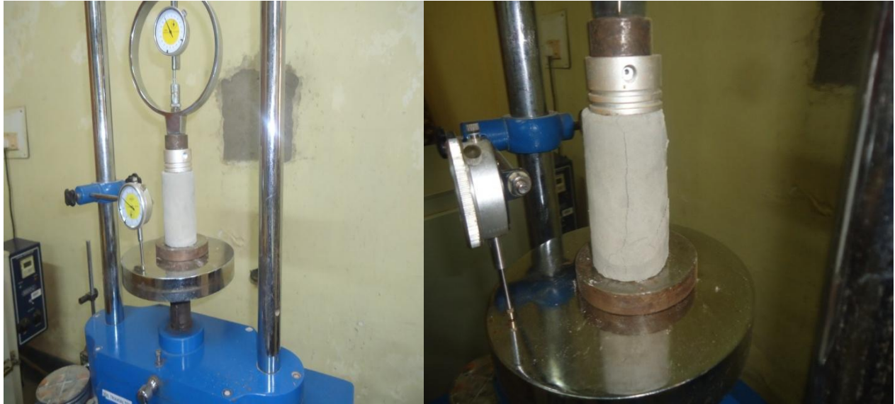
Figure20. Sample testing for UCS
