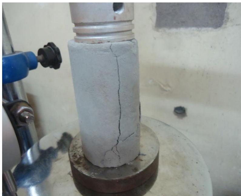
Figure21. Specimen after Failure
