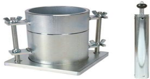
Figure9. Proctor compaction Mould and hammer [28]
