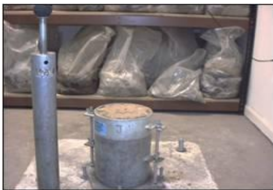
Figure9. Proctor compaction Mould and hammer [28]
