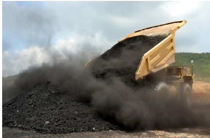
Figure 4.3 Bucyrus MT 4400AC Dump Truck of capacity 240 tons used in the mine
