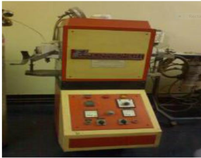
Fig. 3.4.1: High temperature tubular furnace
