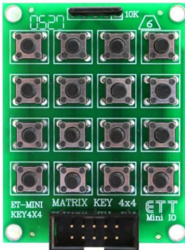
Figure 2.10. 4 x 4 matrix keypad
