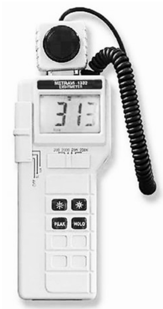
Figure 3.1 Metravi 1332 Digital Lux-meter used for Illumination measurements [31]
