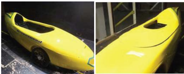
Fig 1.6 Faired vehicles with and without canopy [4]
