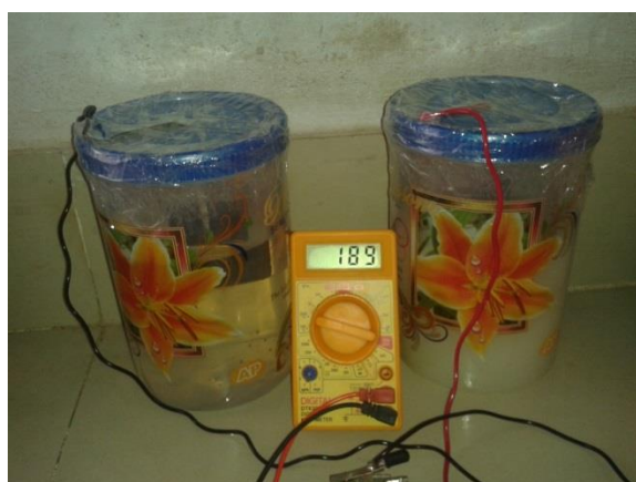
Figure 8:- Voltage and current generated by MFC having chemically treated electrode.
