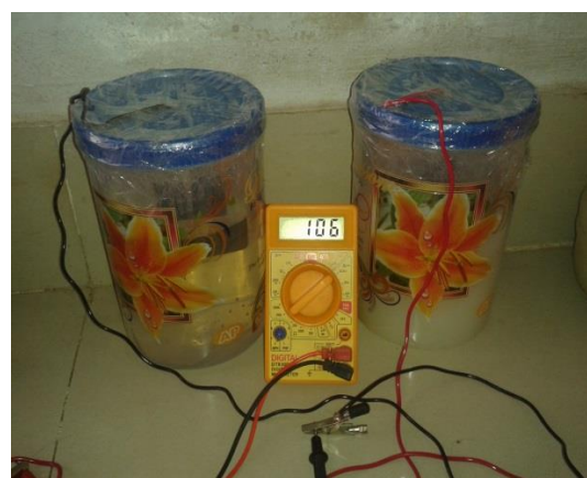
Figure 8:- Voltage and current generated by MFC having chemically treated electrode.
