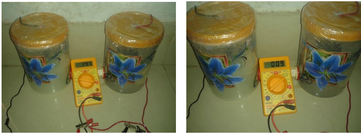
Figure 6:-Voltage & Current generated by Microbial Fuel Cell with increased anode surface area.
