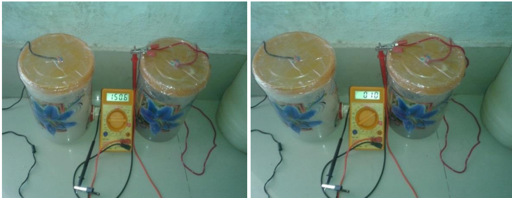
Figure 5- Voltage and Current generated by Microbial Fuel Cell using nanoparticle incorporated salt bridge.
