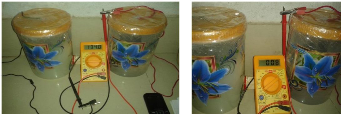
Figure 7:- Voltage and Current generated by MFC having increased cathode surface area
