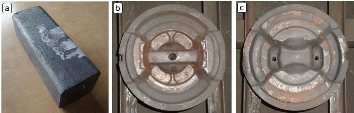
Fig.5.9: Actual set up showing billet and die used for experimental trial a) Input billet material, b) Blocker bottom die, c) Blocker top die
