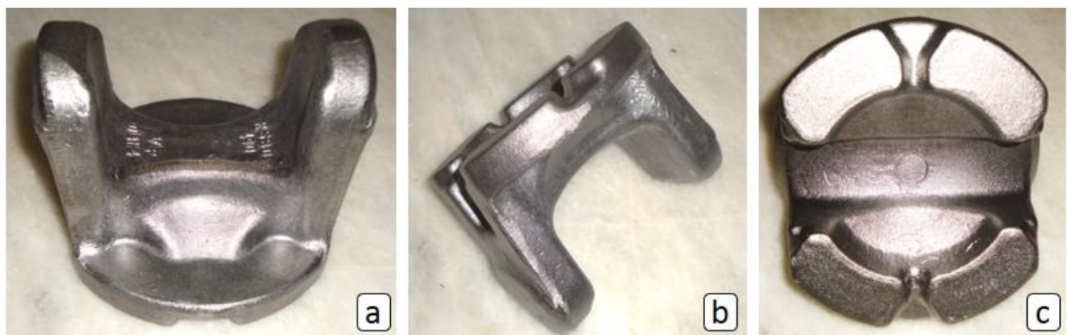
Fig.5.10: a-c Different views of the actual component without flash
