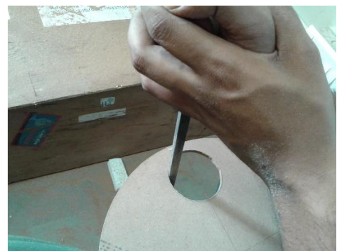
Fig 15: Filing the holes
