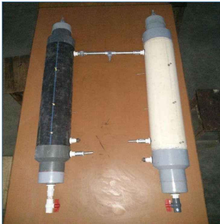
Figure5 Fabricated model of the packed bed scrubber
