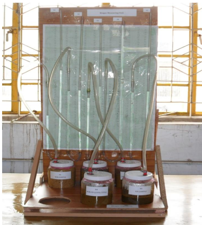
Figure 1 Pictorial view of experimental set up for lab-scale biogas production
