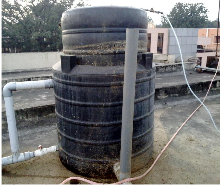
Figure 3 Pictorial view of working model of the floating drum-type biogas digester
