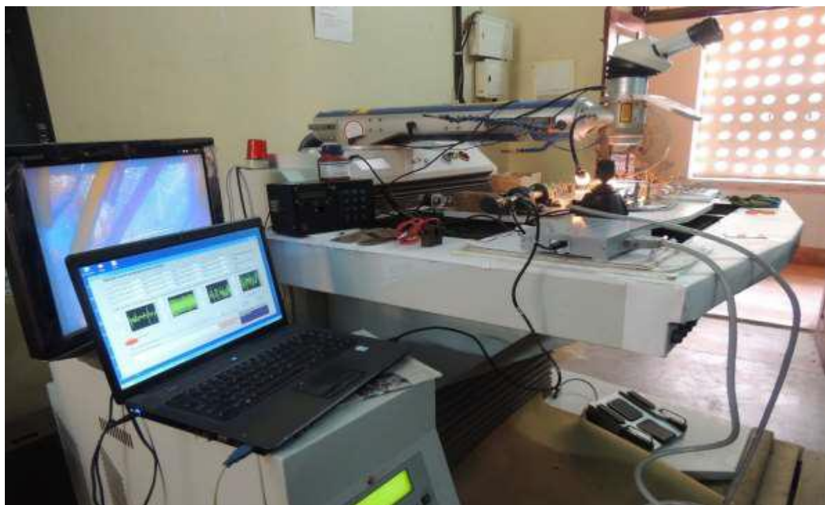
Fig. 9: Pulsed Nd: YAG laser setup
