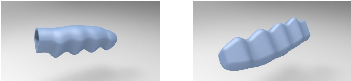
Figure 7.3: Rendered model of tool handle with finger grooves for orientation 1
