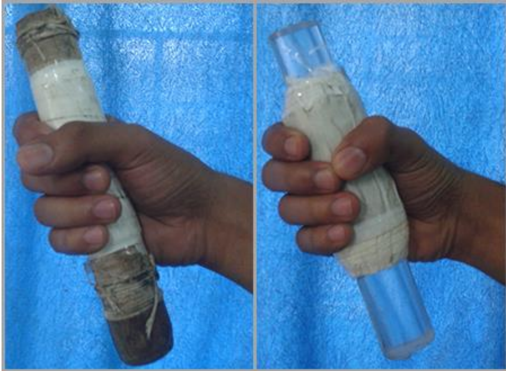
Figure 4.2.1.1: Experimental prototypes used for experimentation to obtain subjective ratings for optimal diameter
