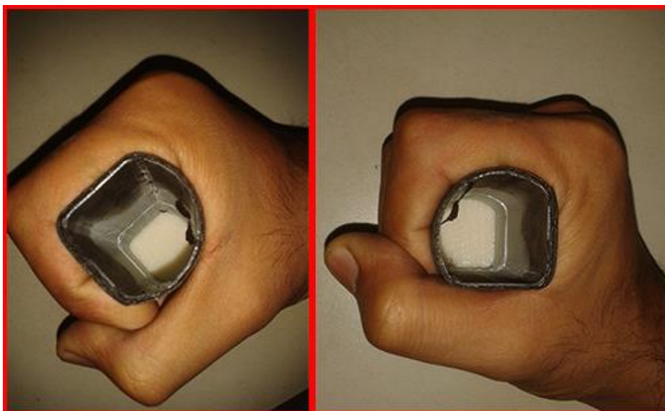
Figure 6.1: The two orientations of tool handle with cross-section of combination of triangle and circle
