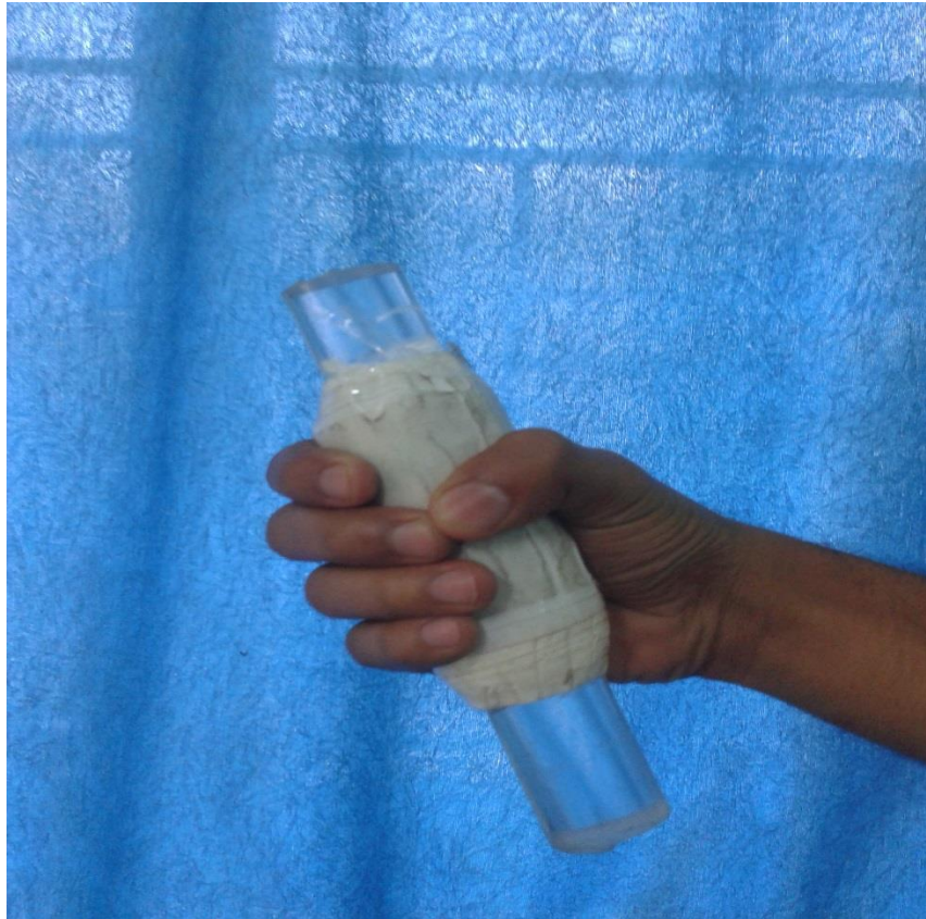
Figure 4.1.6.1: Measurement of grip diameter using padding material
