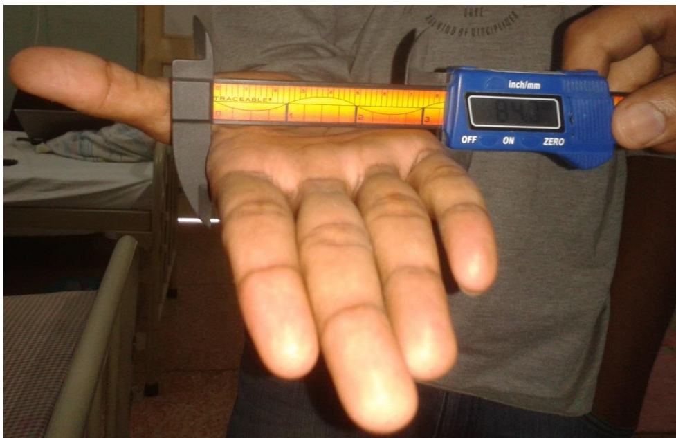
Figure 4.1.2.1: Measurement of Hand breadth
