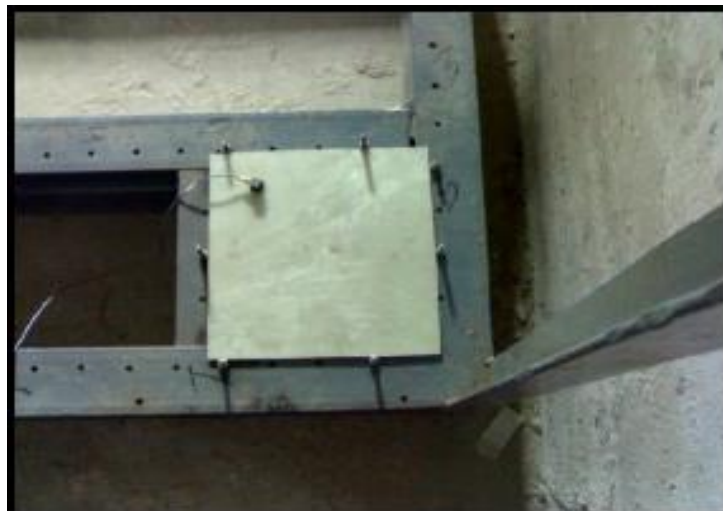
Figure 17: SFSF condition for vibration testing.
