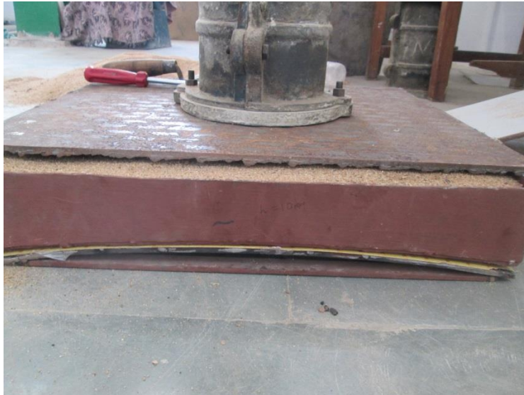
Figure 8: Parallel view of shell and mould during curing
