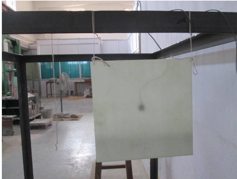
Figure 16: FFFF condition for vibration testing
