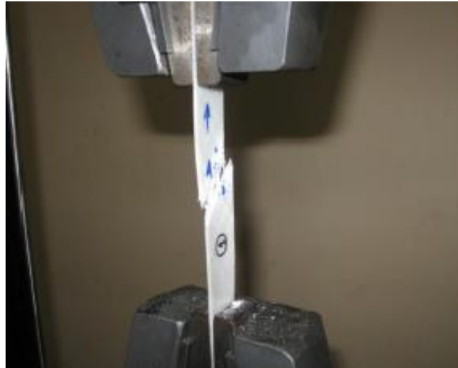
Figure 6: Failure pattern of tensile test specimen
