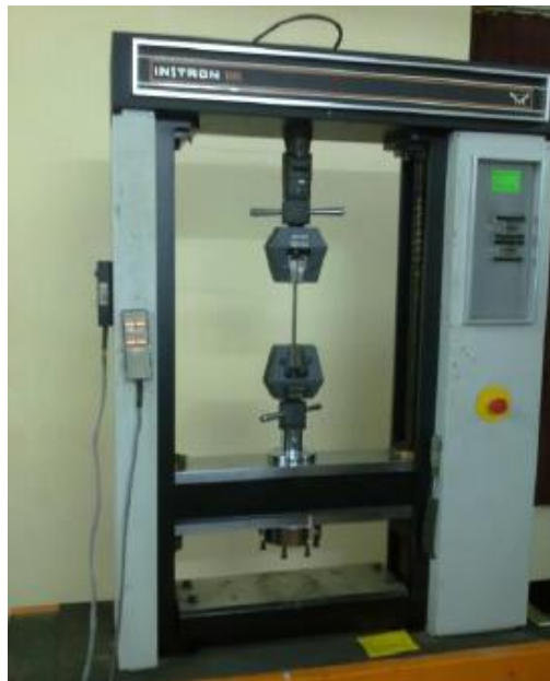
Figure 5: Tensile test setup in INSTRON 1195 UTM machine
