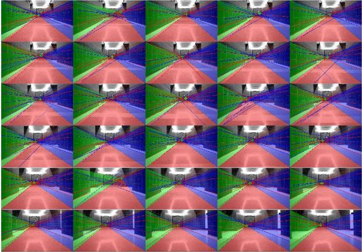
Fig 6.3 Detected Vanishing Point and the corresponding planar segmentation
