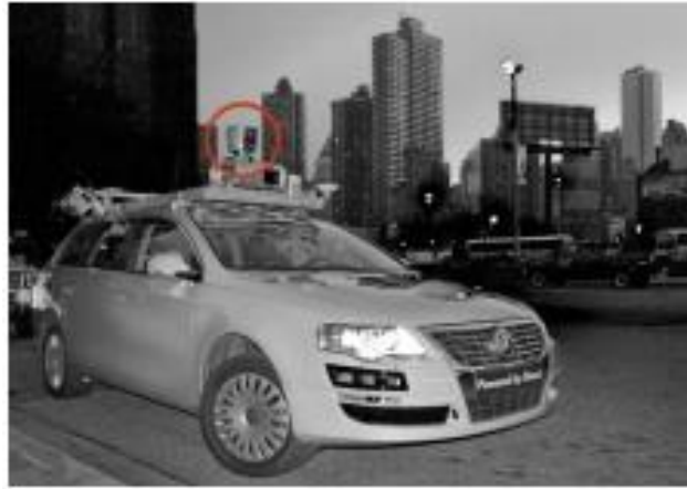
Fig 1.4 Stanford's Junior with a surmounted Velodyne HD-LIDAR 64-beam scanner is circled in red.
