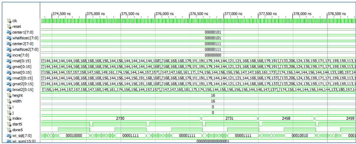
Figure 4. 7 VHDL simulation showing the values for weight matrix
