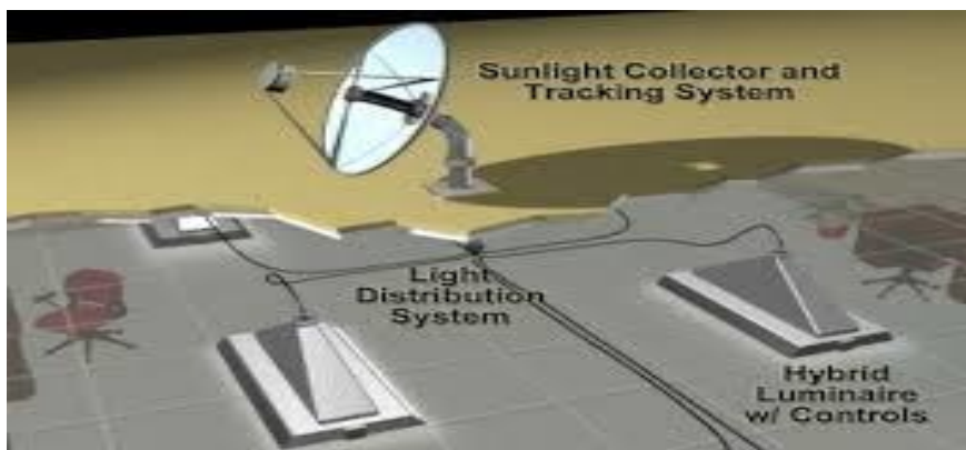
Figure3.4 Hybrid Solar Lighting System
