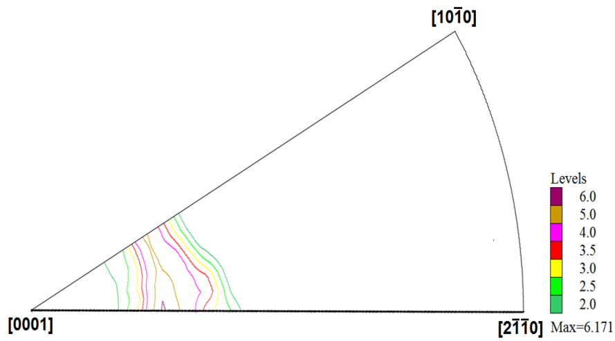
Figure 23 Inverse pole figure showing bulk texture of sample oriented towards the rolling direction
