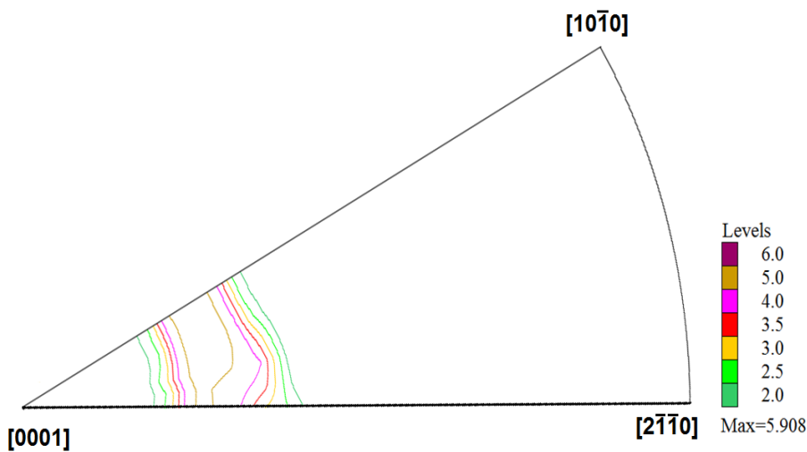
Figure 25 Inverse pole figure showing bulk texture of sample oriented 90 deg to the rolling direction
