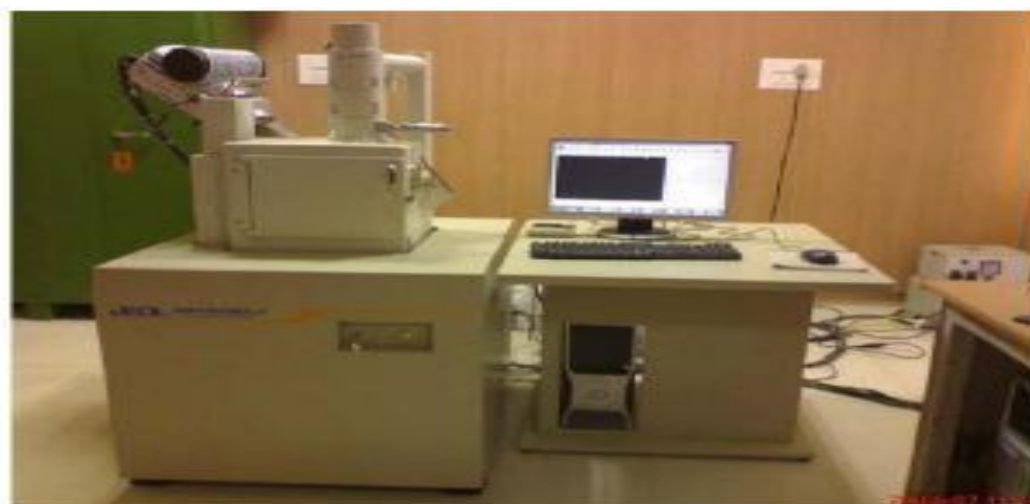
Figure: 3.4 Scanning Electron Microscope (JEOL-JSM 6480 LV SEM)
