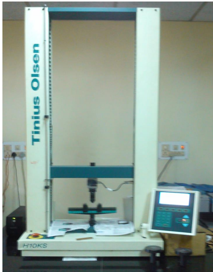
Figure.3.2: Loading arrangement for three point bending test
