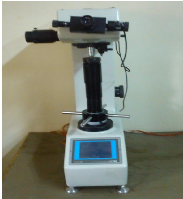
Figure.3.3: Experimental set up for Micro-hardness test
