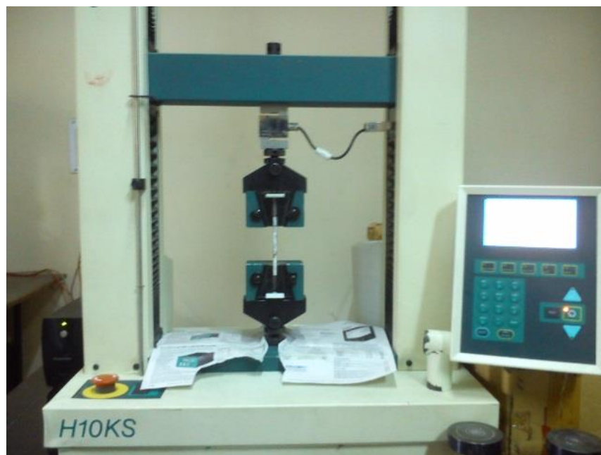
Figure.3.1: Loading arrangement for tensile test
