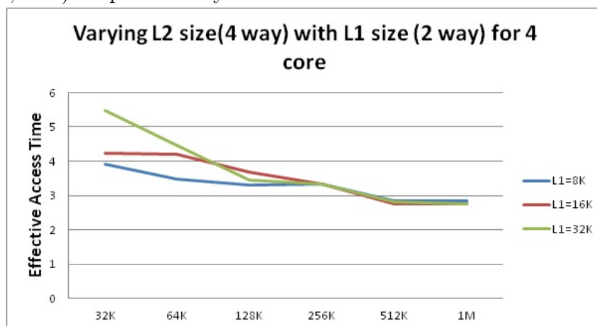
Figure 3.11: Effective access time on executing FFT for L1 cache sizes (8kb,16kb,32kb) in quad core system
