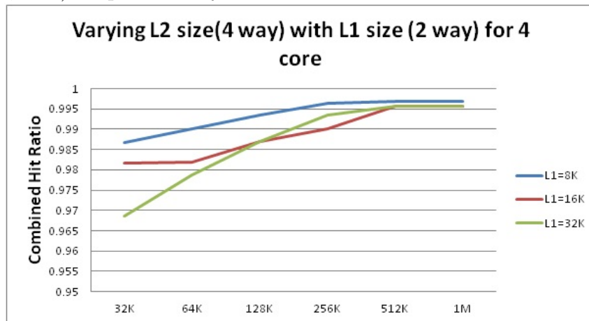
Figure 3.10: Combined hit ratio on executing FFT for L1 cache sizes (8kb,16kb,32kb) in quad core system
