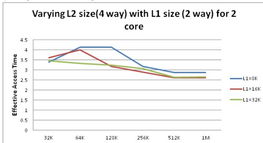
Figure 3.8: Effective access time on executing FFT for L1 cache sizes (8kb,16kb,32kb) in dual core system
