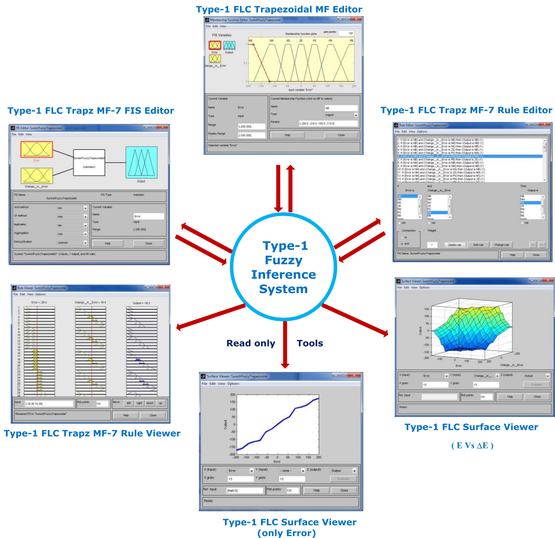
Fig. 3.11 (a) Type-1 Fuzzy Inference System with Trapezoidal MF 7x7
