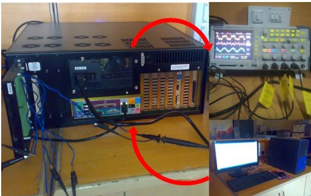
Fig. 2.15 Real-time implementation of Shunt active filter control strategies using OPAL – RT
