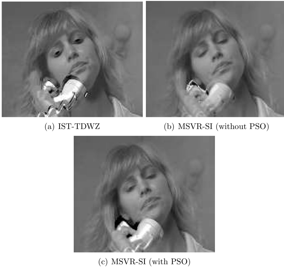
Figure 5.8: Subjective analysis of a decoded SI frame (36 th frame of Suzie )
