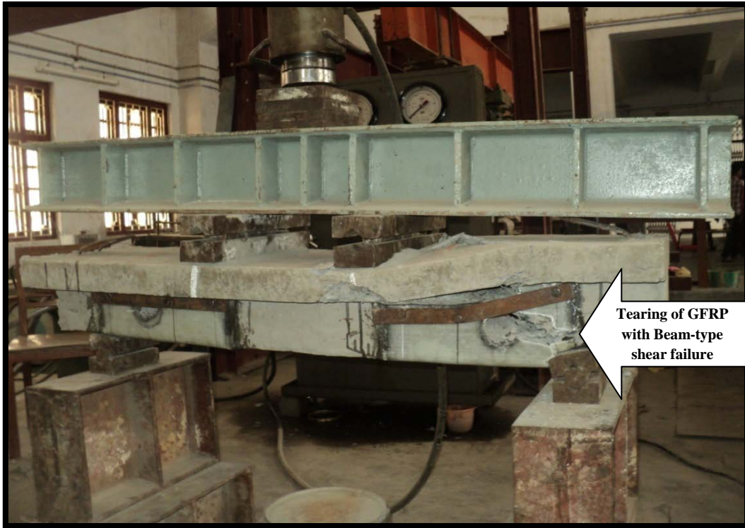
(c) Crack Pattern of SB12
