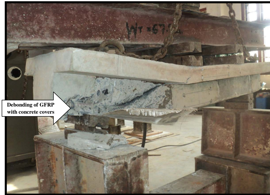
(c) Complete debonding followed by shear failure
