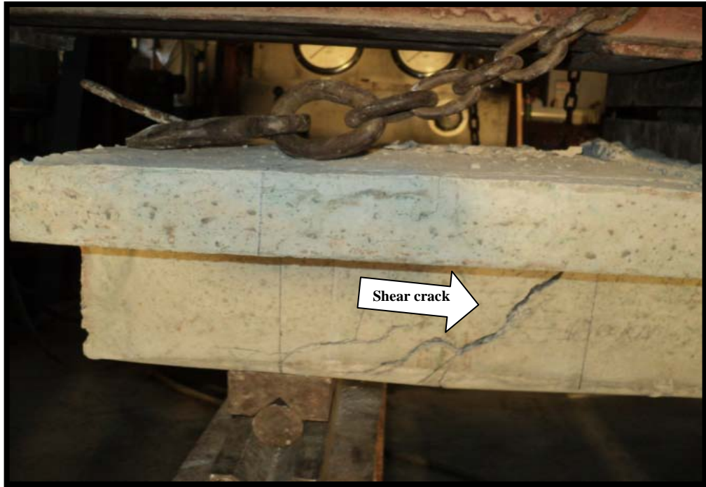
(c) Crack Pattern at L/3 distance (Near Left Support)
