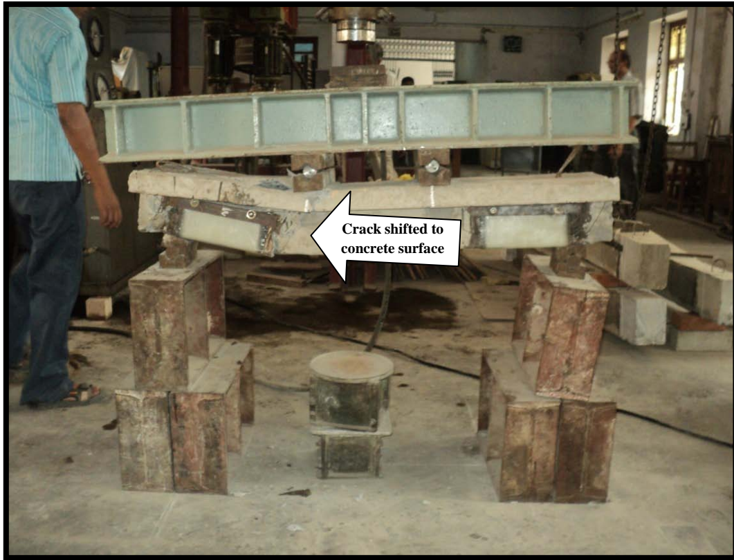
(b) Crack shifted to the un-strengthened part of the shear span
