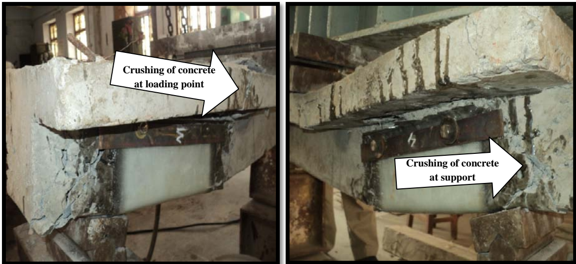
(c) Crushing of concrete near the support and the loading point
