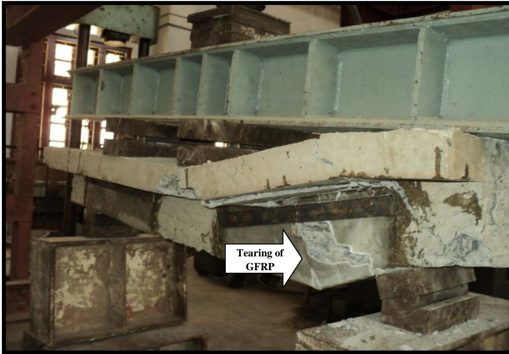
(b) Magnified view of Tearing of GFRP
