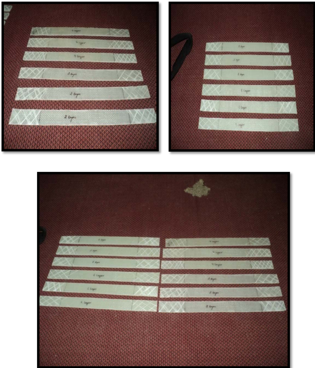
Figure 3-3. Specimens for tensile testing of woven Glass/Epoxy composite
