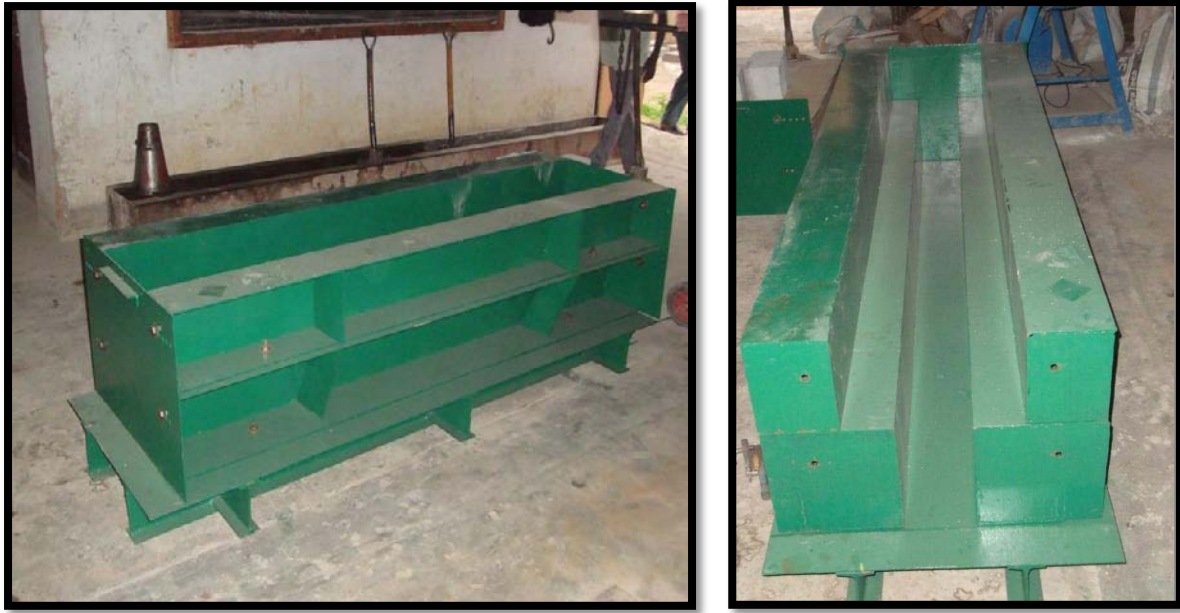
Figure 3-6. Steel Frame Used For Casting of RC T-Beam
