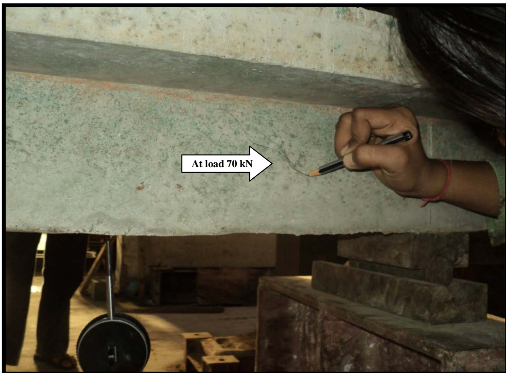
(b) Hair line crack started at 70kN in shear region
