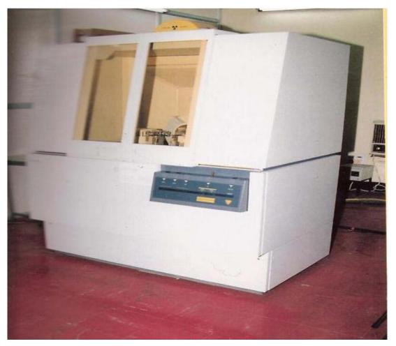
Fig. 4.6 Philips X-pert MPD X-ray diffractometer.
