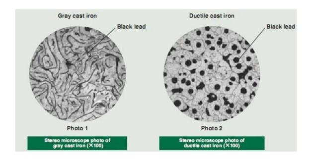
Fig. 2.8 microstructure of gray and ductile iron[53]
