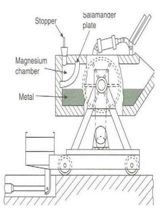
Fig.1.2 G.F. Fisher Method for production of ductile iron [7].
