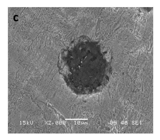
Fig.5.33 Microstructure of the austempered ductile iron (Nickel alloyed) austempered at (a) 250°C for 60 min (b) 300°C for 60 min (c) 350°C for 60 min
