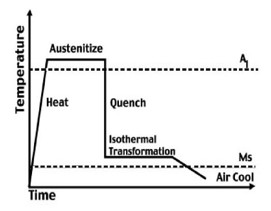
Fig.2.12 Austempering process [17].
