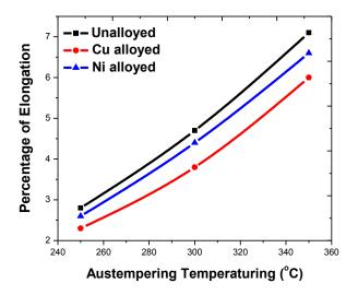
Fig. 5.20 Effect of austempering temperature on Elongation for 120 min
