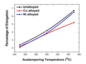
Fig. 5.18 Effect of austempering temperature on Elongation for 60 min
