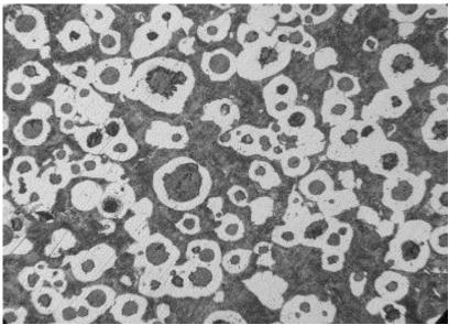
Fig. 2.5 Representative pearlitic ductile iron microstructure [46].
