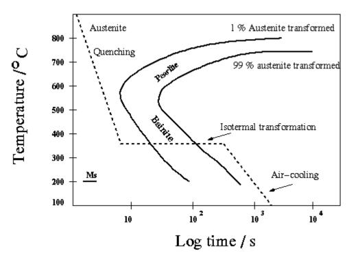
Fig. 2.4 Diagram for austempering superimposed on TTT diagram
