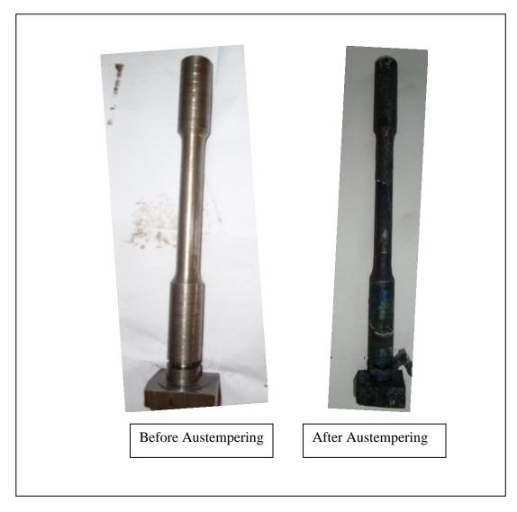
Fig. 4.2 Dog bone shaped ductile iron before and after austempering
