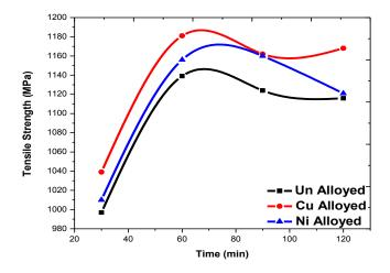
Fig. 5.4Effect of austempering time on UTS, austempered at 250 °C
