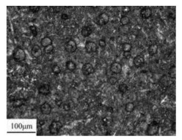
Fig. 2.9 Microstructures of ductile cast iron with the addition of nickel [14].
