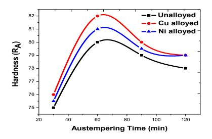
Fig. 5.10 Effect of austempering time on hardness, austempered at 250 °C
