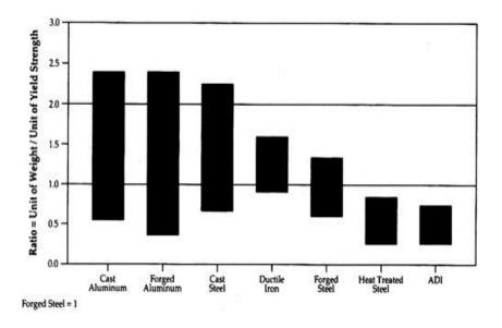
Fig. 2.16Less weight compared to the other steels [20].
