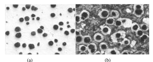
Fig 2.3.Mirostructure of ductile iron (a) unethed (b) nital etched :100X [22].
