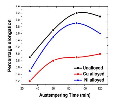
Fig. 5.9Effect of austempering time on elongation, austempered at 350 °C
