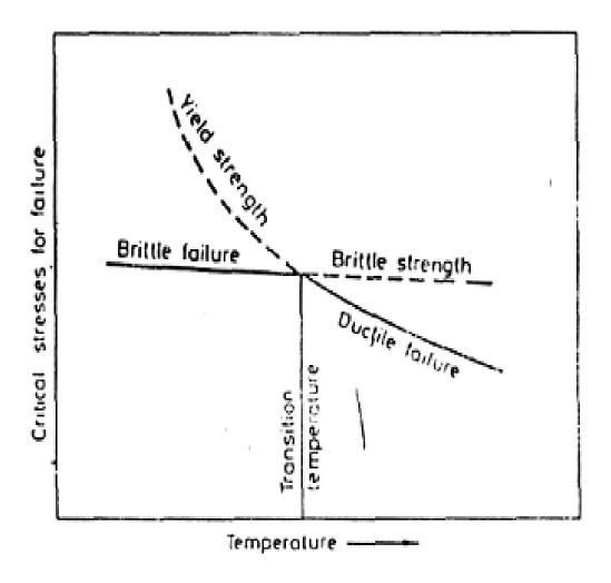
Fig.2.11 Ductile to Brittle transition occurs as temperature increases [16].
