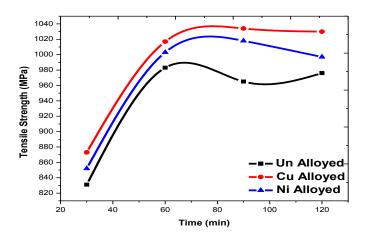
Fig. 5.5 Effect of austempering time on UTS, austempered at 300 °C
