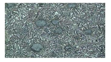
Fig. 2.14 Microstructure of austempered ductile iron [24]
