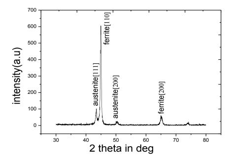
Fig.5.27 XRD pattern of ductile iron austempered at 350°C for 60 min.
