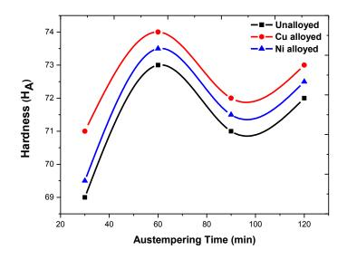
Fig. 5.11 Effect of austempering time on hardness, austempered at 300 °C
