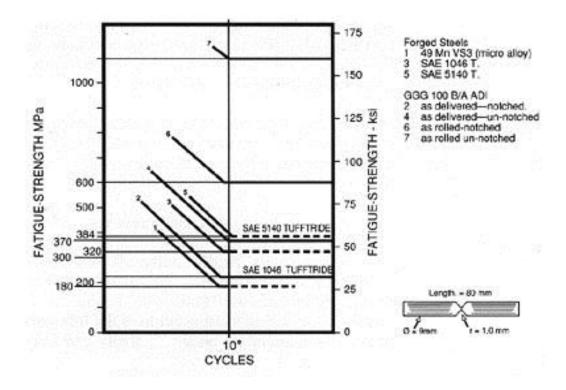
Fig. 2.15Fatigue strength compared to other materials [20].
