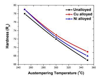
Fig.5.24 Effect of temperature on hardness for 120 min
