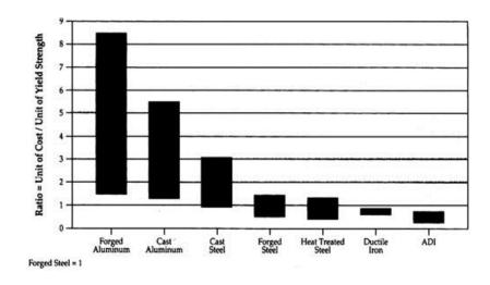
Fig. 2.17Relative cost per unit of yield strength [20]
