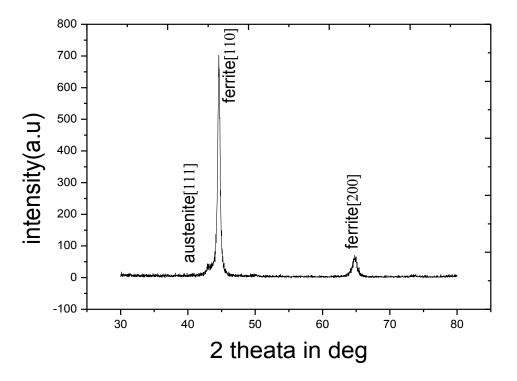
Fig.5.30 XRD pattern of alloyed ductile iron austempered at 300°C for 60 min.
