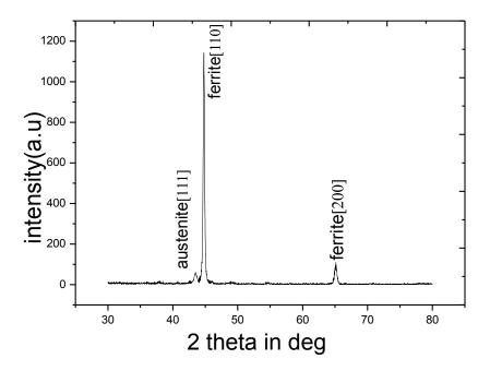
Fig.5.25 XRD patterns of ductile ironsample austempered at  $250^{\circ}$ C for (a) 60 min and (b) for 90 min.
