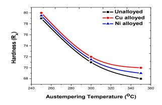
Fig. 5.23 Effect of temperature on hardness for 90 min
