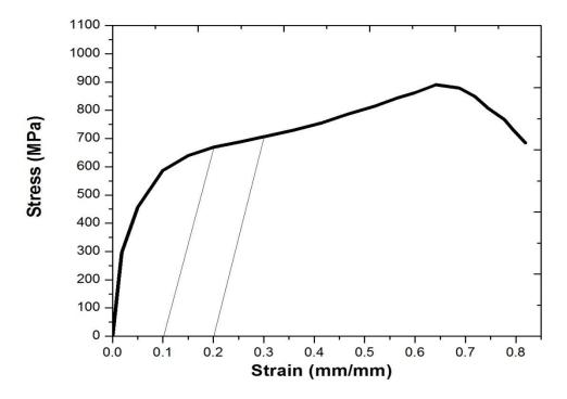
Figure 5.3 Stress-strain curve of Ni-alloyed ADI austempered at 350 °C for 90 min.
