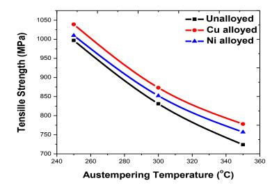
Fig. 5.13 Effect of austempering temperature on UTS for 30 min
