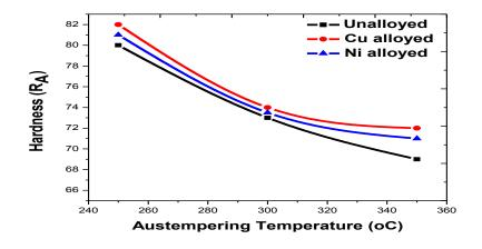
Fig. 5.22 Effect of temperature on hardness for 60 min
