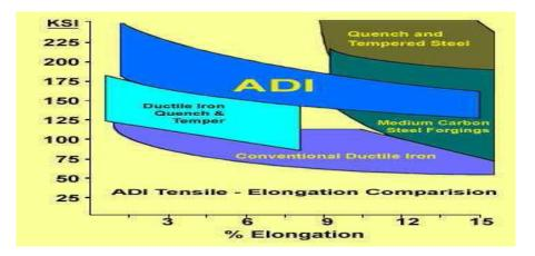
Fig. 2.18Properties of ductile iron compared steels [25].
