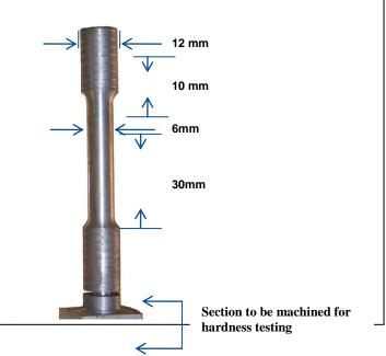
Fig. 4.1 Test Specimen
