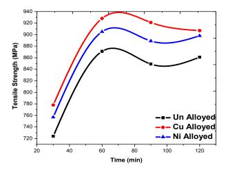
Fig. 5.6Effect of austempering time on UTS, austempered at 350 °C
