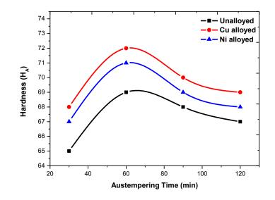
Fig. 5.12 Effect of austempering time on hardness, austempered at 350 °C
