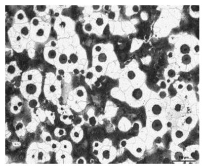
Fig. 2.7Ferritic-pearlitic ductile iron microstructure (Nital 3 %) [48].
