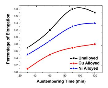
Fig. 5.8Effect of austempering time on elongation, austempered at 300 °C
