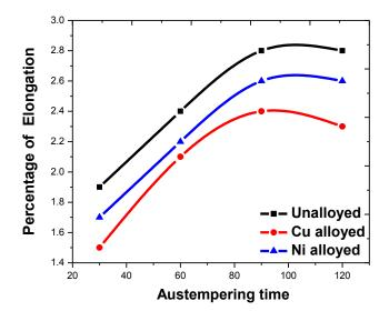
Fig. 5.7Effect of austempering time on elongation, austempered at250 °C
