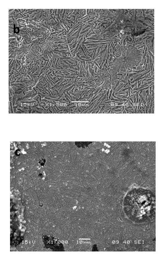
Fig.5.32 Microstructure of the austempered ductile iron (Copper alloyed) austempered at (a) 250°C for 60 min (b) 300°C for 60 min (c) 350°C for 60 min
