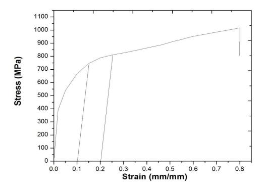
Figure 5.2 Stress-strain curve of Cu-alloyed ADI austempered at 300 °C for 60 min.
