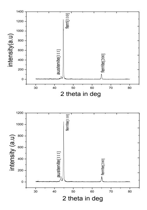
Fig.5.26 XRD patterns of ductile iron austempered (a) at 250°C for 120 min and (b) at  $300^{\circ}$ C for 60 min.
