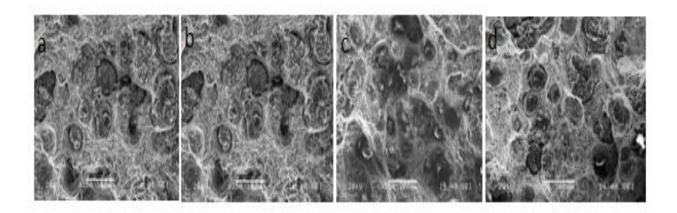
Fig. 5.34 Fracture surfaces of the copper alloyed ductile iron which is austempered at 250°C for (a) 30 min (b) 60 min (c) 60 min (d) 120 min
