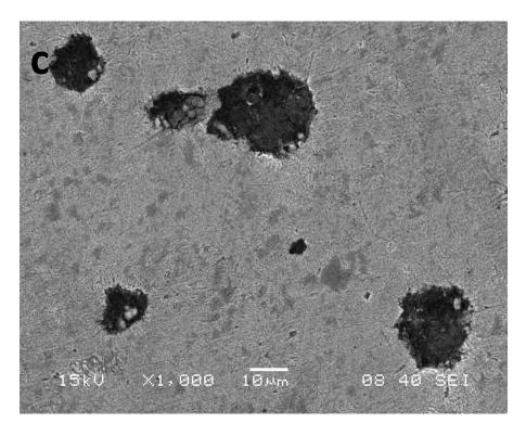
Fig. 5.31 Microstructure of the austempered ductile iron (unalloyed) austempered at (a) 250°C for 30 min (b) 350°C for 60 min (c) 300°C for 60 min
