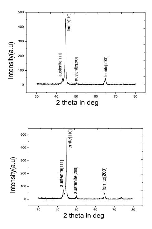
Fig.5.29XRD patterns of alloyed ductile iron austempered at 250°C for 30 min and 350°C for 60 min.
