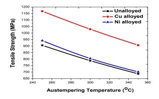
Fig. 5.16 Effect of austempering temperature on UTS for 120 min
