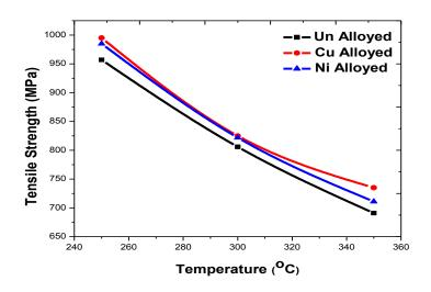
Fig. 5.14Effect of austempering temperature on UTS for 60 min
