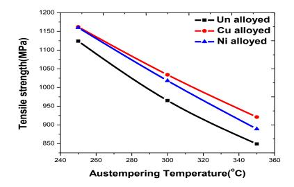
Fig. 5.15 Effect of austempering temperature on UTS for 90 min
