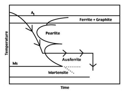
Fig.2.13 Control of time and temperature on the process [18].
