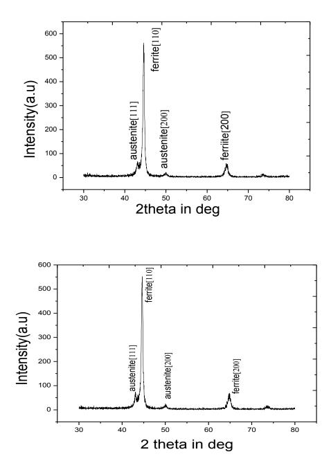
Fig.5.28 XRD patterns of alloyed ductile iron austempered at 250°C for 60 min and 120min.
