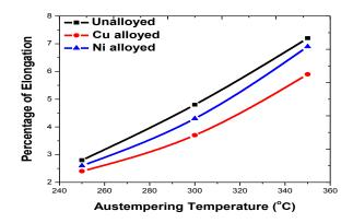
Fig. 5.19 Effect of austempering temperature on Elongation for 90 min
