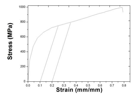
Figure 5.1 Stress-strain curve of unalloyed ADI austempered at 250 °C for 30 min.
