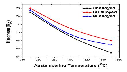
Fig. 5.21 Effect of temperature on hardness for 30 min
