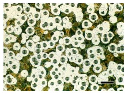
Fig. 2.6Pearlitic-ferritic matrix of a ductile iron after etching with 4% Nital[47].
