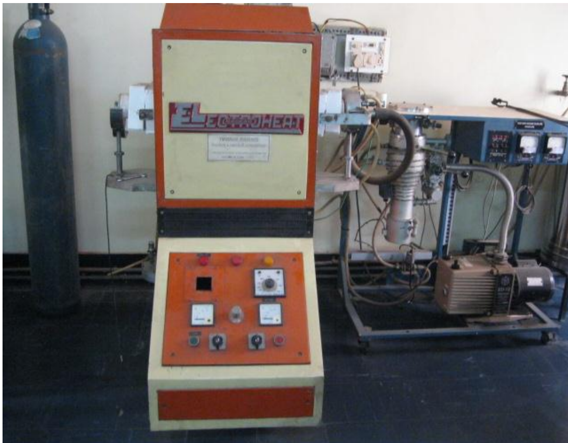
Fig. 3.3: Horizontal Tubular Furnace
