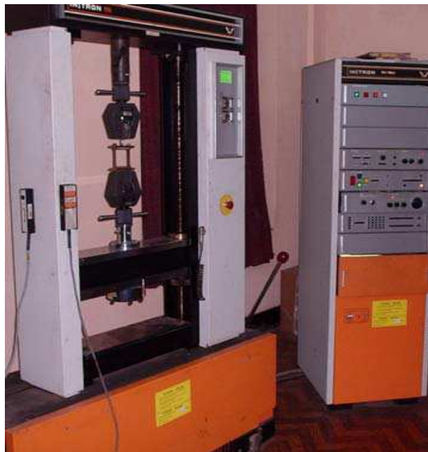
Figure 3.3 Experimental set up for tensile test
