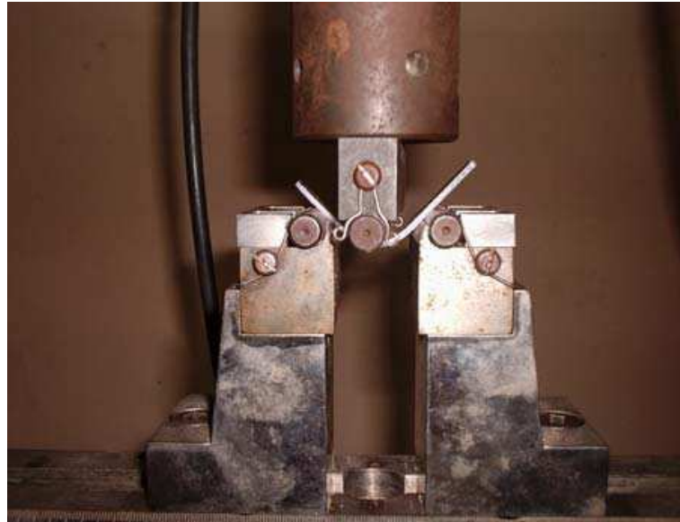
Figure 3.5 Loading arrangement for flexural test
