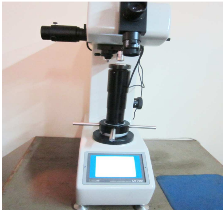
Figure 3.6 Experimental set up for Micro-hardness test
