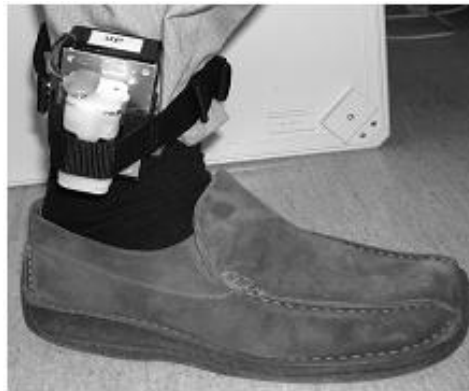
Figure 1.3 : The MR sensor attached to the lower leg [6].
