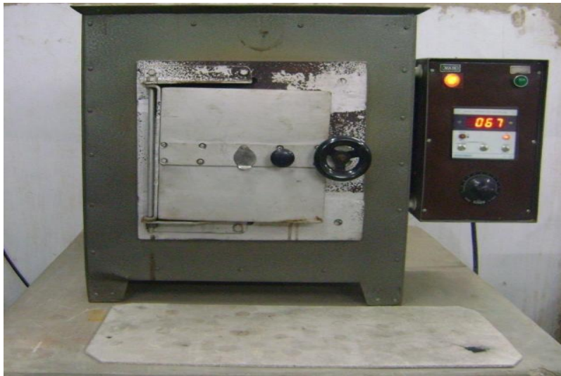
Plate 3.2 Muffle Furnace for Determination of Volatile Matter and Ash Content
