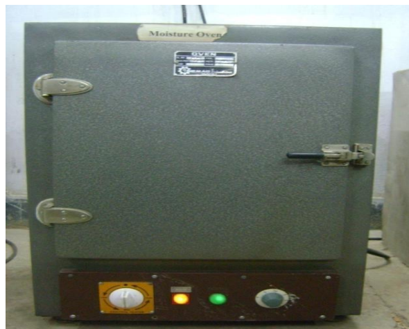
Plate 3.1 Oven for Moisture Content Determination
