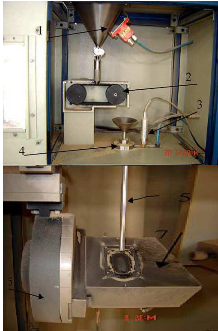
Fig.-3.1 Details of erosion test rig. (1) Sand hopper, (2) Conveyor belt system for Sand flow, (3) Pressure transducer, (4) Particle-air mixing chamber, (5) Nozzle, (6) X–Y and h axes assembly, (7) Sample holder.
