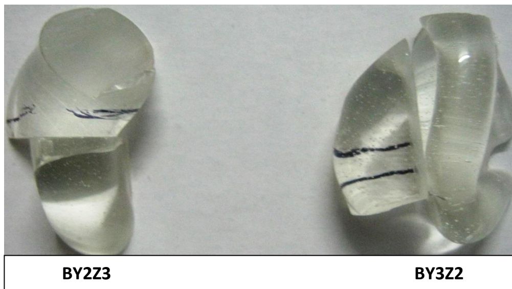
Figure No 4: Base glasses containing \text{ZrO}_2 as nucleating agent
