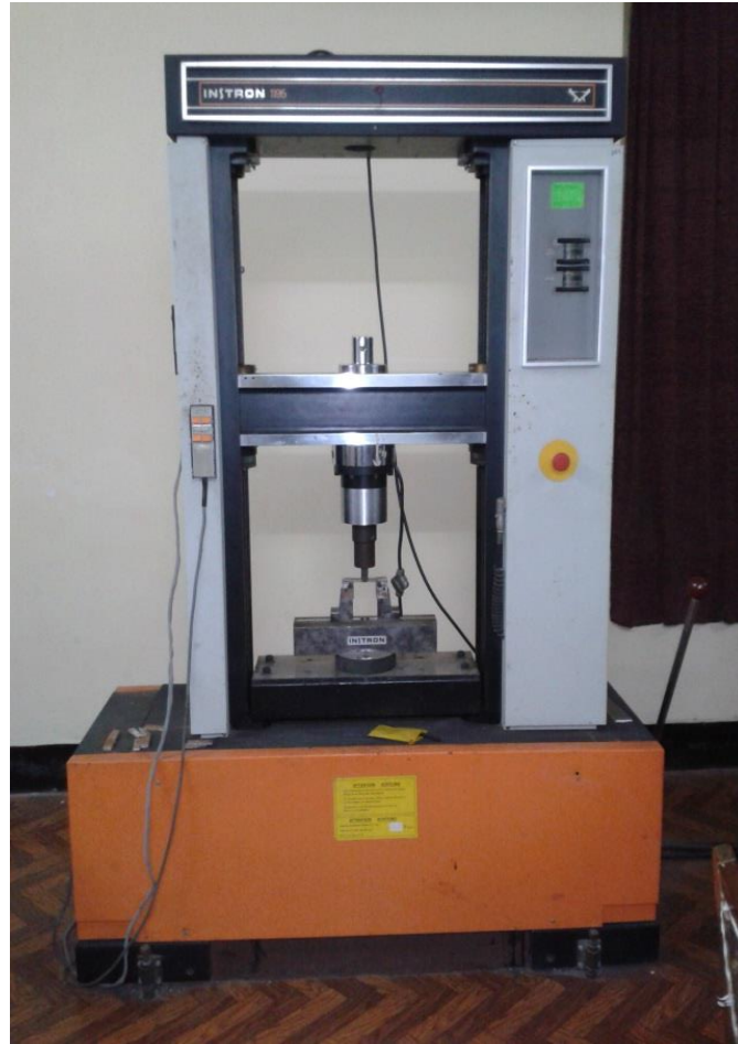
Figure 3.5 Experimental set up and loading arrangement for the specimens for three points bend test
