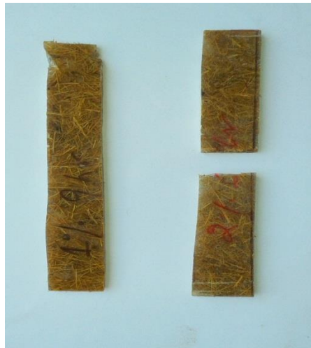
Figure 3.4 Flexural Test Specimens
