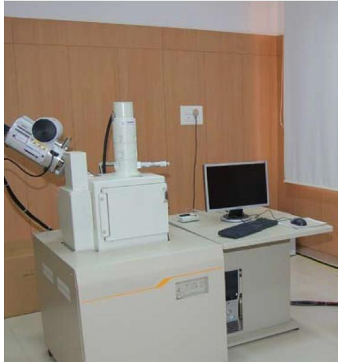
Figure 3.6 Scanning electron microscope set up.
