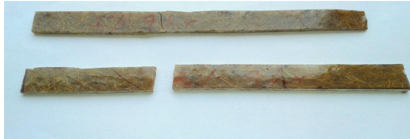
Figure 3.3 Tensile Test Specimens
