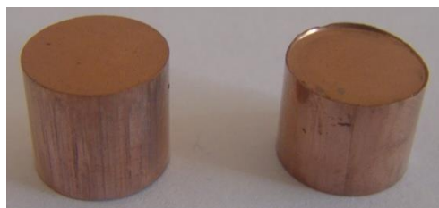
Figure 6 : P/M compacted tool electrode tips
