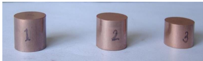
Figure 9 : P/M compacted tool electrode tips prepared with various % of W and Cu and with different compact pressure
