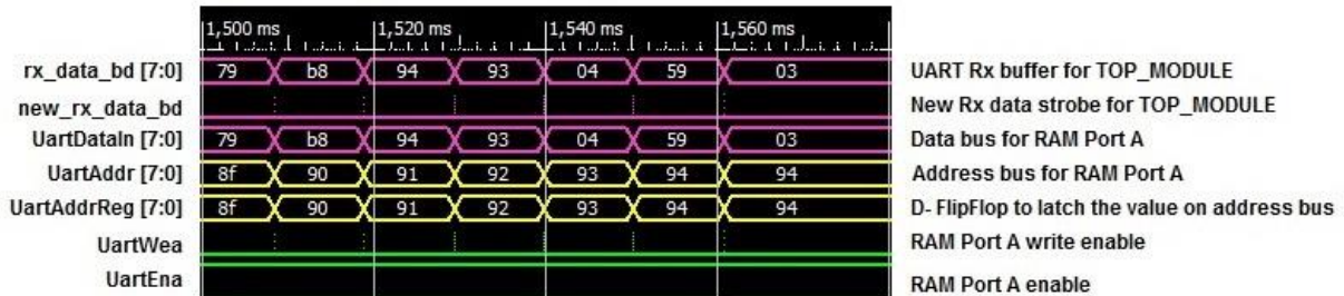
Figure 16 Waveforms depicting signals involved in transfer of data from UART to BRAM
