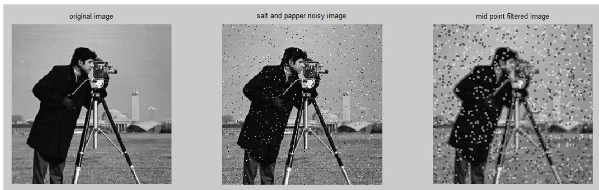
fig 4.7: (a)Original image (b)Image with salt and pepper noise (c)Mid point filtered image
