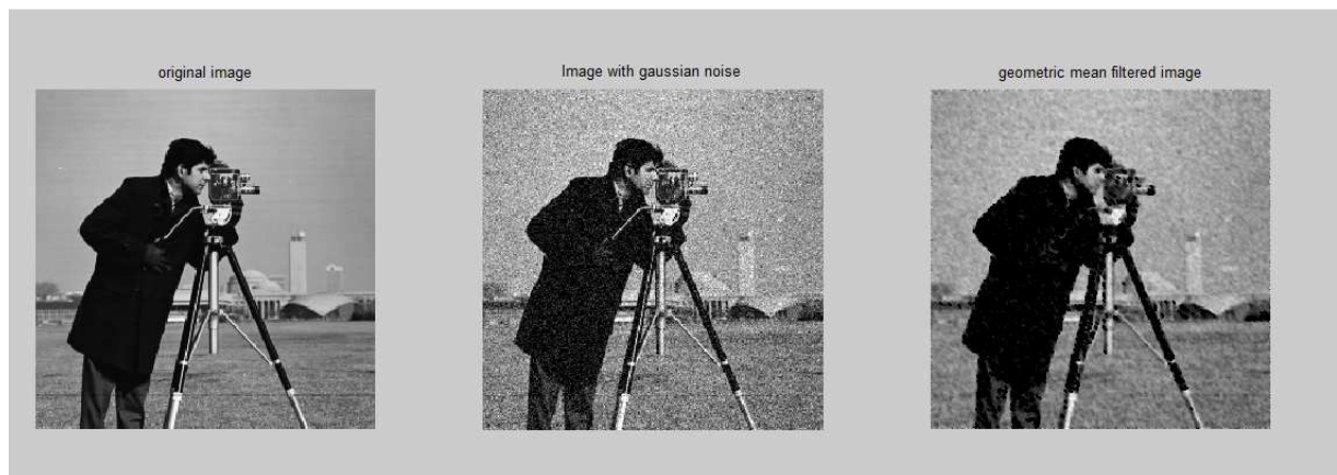
fig 4.2: (a)Original image (b)Image with gaussian noise (c)Geometric mean filtered image.
