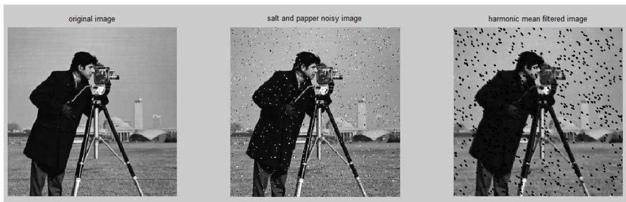
fig 4.3: (a)Original image (b)Image with salt and pepper noise (c)Harmonic mean filtered image
