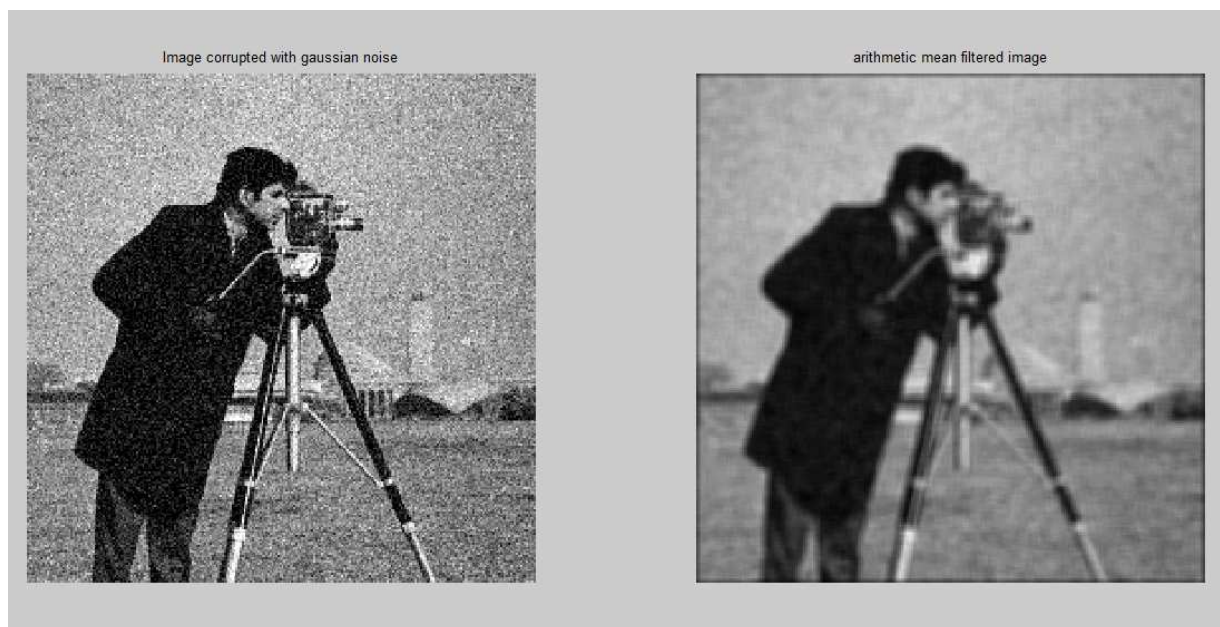
Fig 4.1: (a) Image corrupted with Gaussian noise (b) Arithmetic mean filtered image
