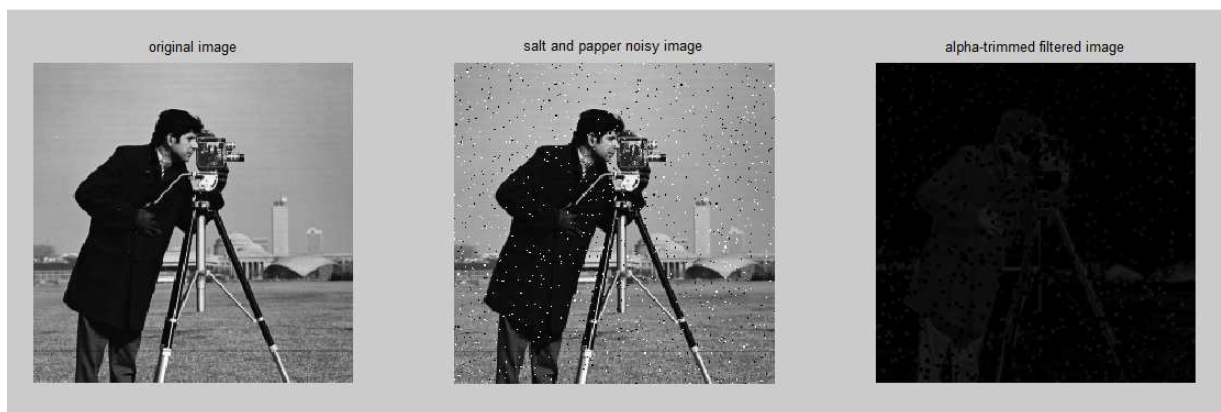
fig 4.8: (a)Original image (b)Image with salt and pepper noise (c)Alpha-trimmed filtered image
