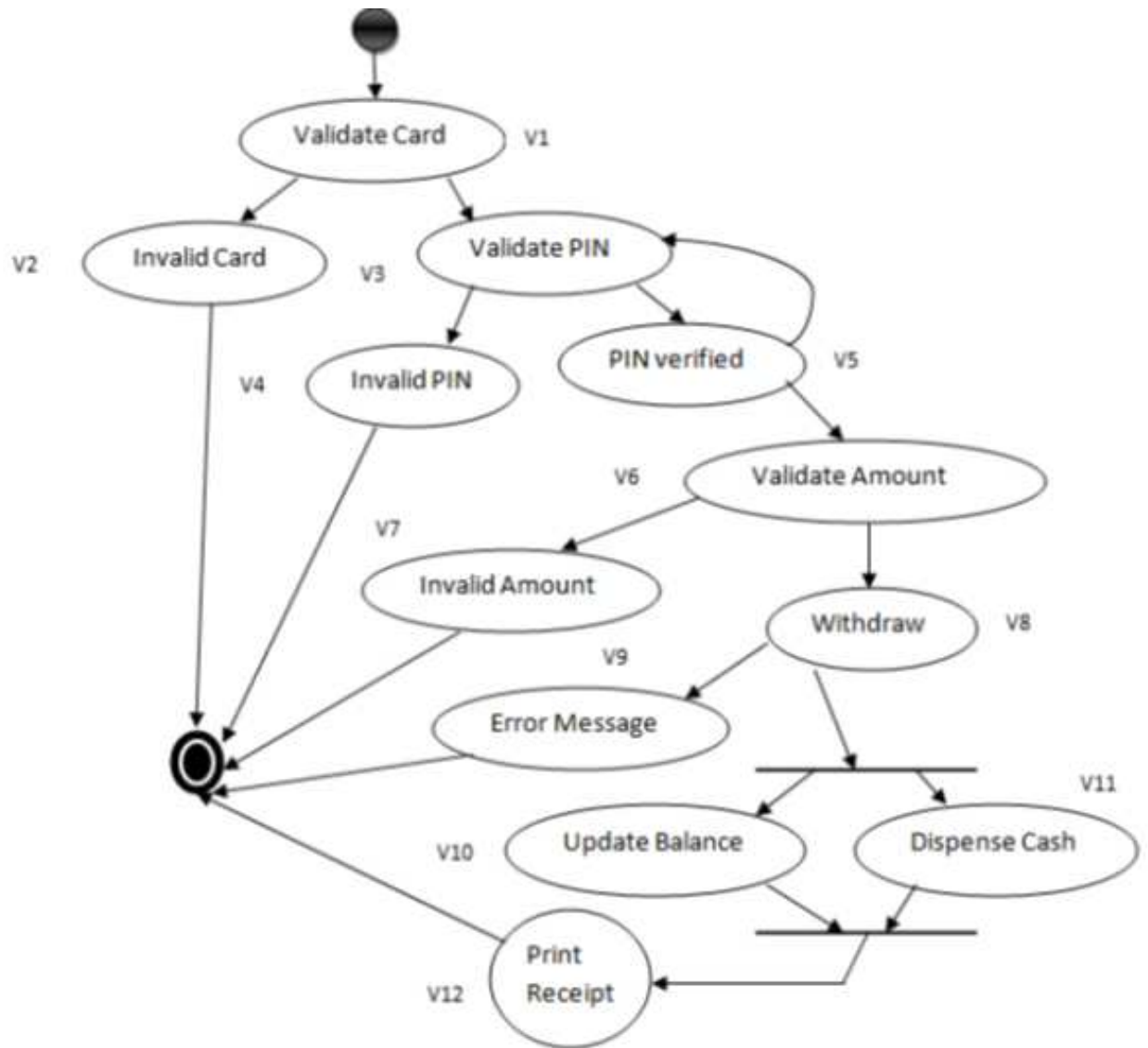
Figure 5.7: UML Interaction Graph (UIG) for ATM withdraw use case
