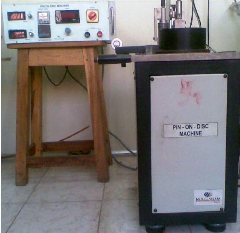
Fig-2: set up for study of abrasive wear of sample
