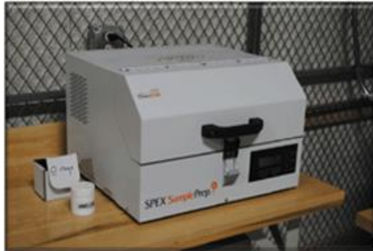
Figure 3.1: Spex 8000M Ball Mill, (Zirconia & Steel mill sets)
