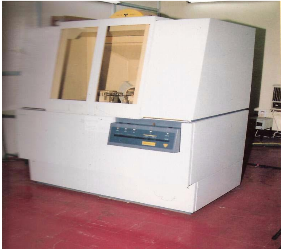
Figure 3.2: Philips X-pert MPD X-ray diffractometer.
