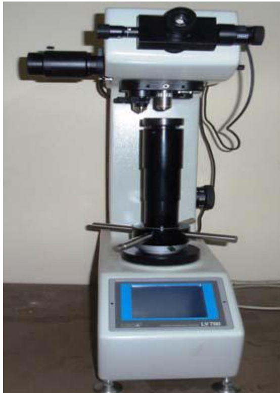
Figure 3.4: Leco LV 700 Vickers hardness tester
