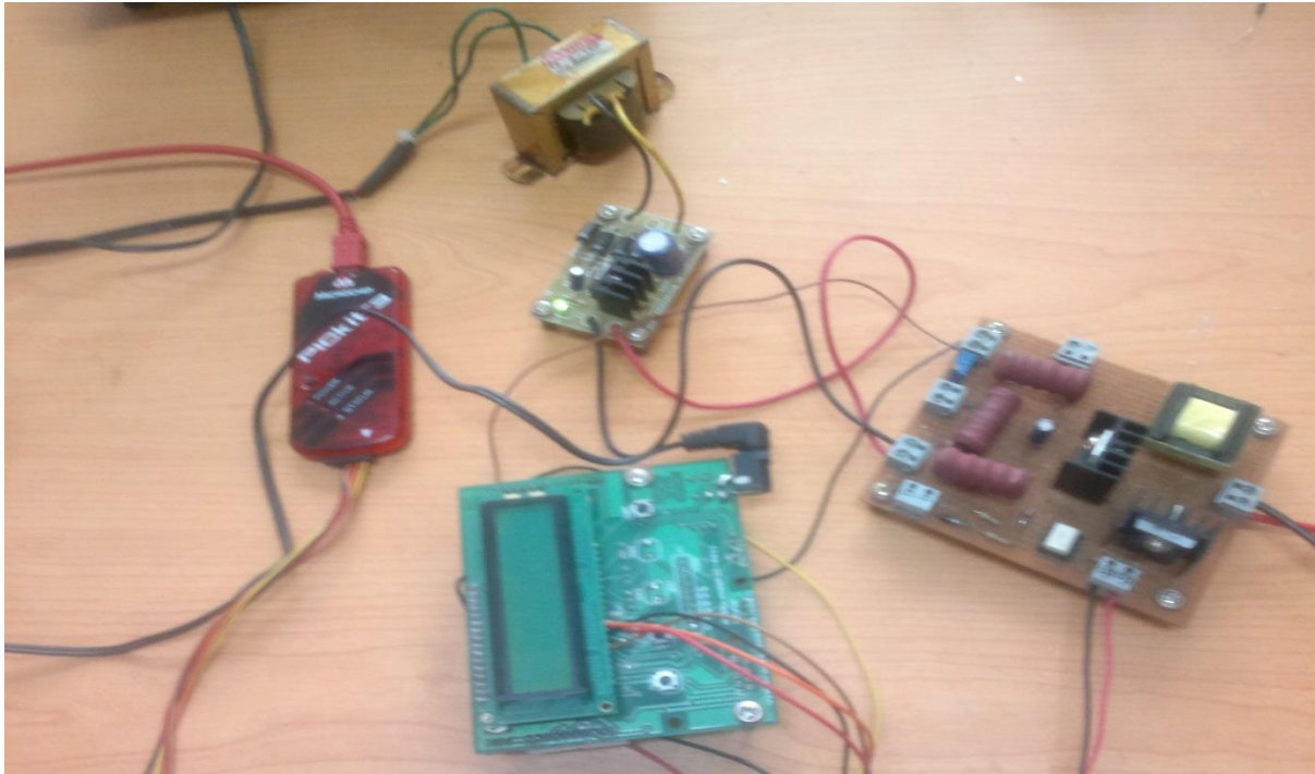
Fig 4.7 model of buck converter with microcontroller
