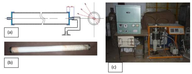
Fig. 3.3: CAD drawing (a) and photograph (b) of the attachments made for attaining vacuum in tubular furnace (c).
