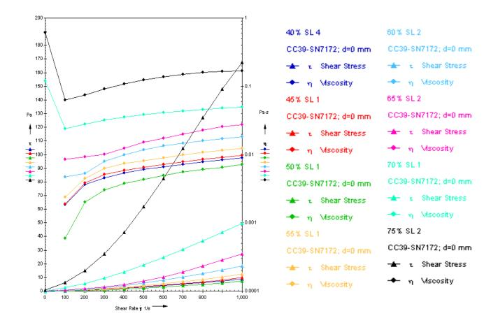
Fig. 4.3: Variation kinematic viscosity and shear stress with respect to strain rate of colloidal solution having alumina powder with different solid loading.
