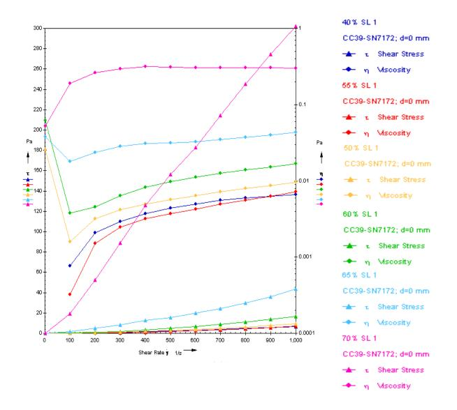
Fig. 4.2: Variation kinematic viscosity and shear stress with respect to strain rate of colloidal solution having aluminium powder with different solid loading.
