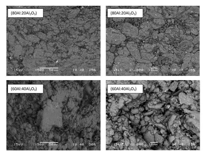
Fig. 4.17: SEM images of 80Al:20Al<sub>2</sub>O<sub>3</sub> and 60Al:40Al<sub>2</sub>O<sub>3</sub> composites.
