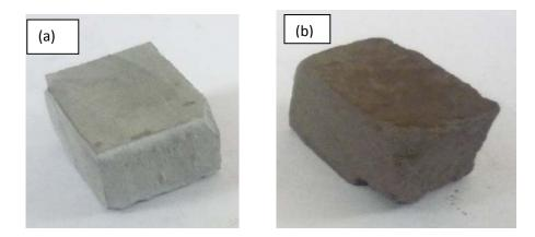
Fig. 4.8 (a) and (b) shows the green and fired gelacted product.
