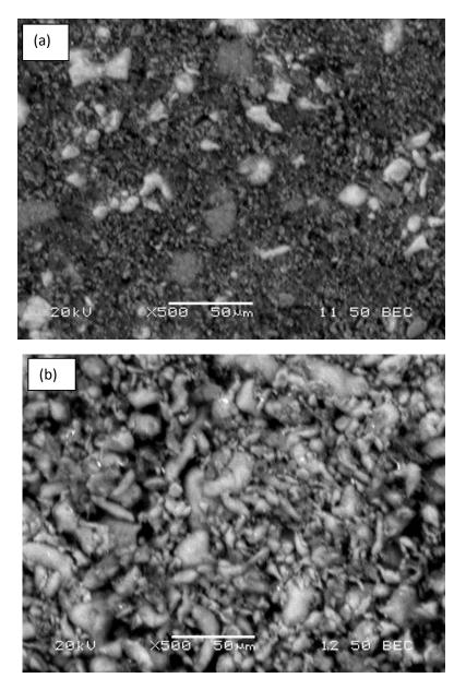
Fig. 4.9: SEM image of (a) green body and (b) sintered Al-Al<sub>2</sub>O<sub>3</sub> product made by gelcasting.
