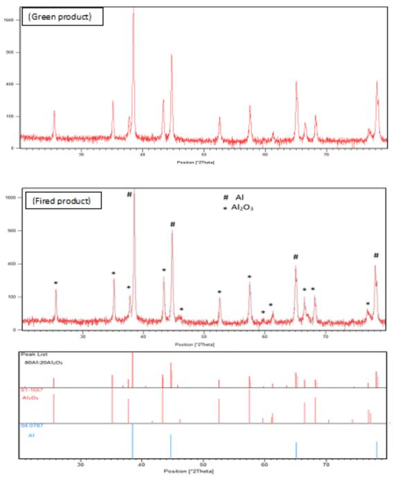
Fig. 4.10: XRD pattern of green 80Al-20Al<sub>2</sub>O<sub>3</sub> product and fired product.
