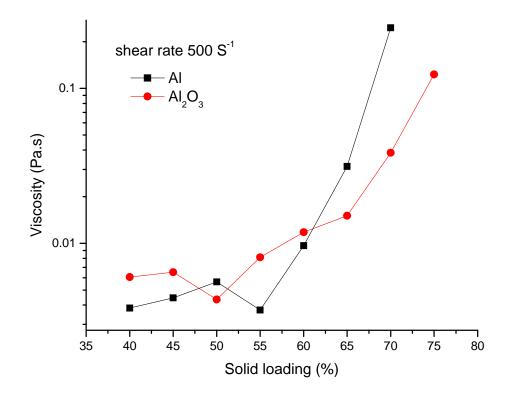
Fig. 4.4: Variation of viscosity with respect to the solid loading of both alumina and aluminium powder.
