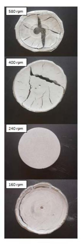
Fig. 4.6: Image of green gelcasted body after drying prepared through at different rpm.
