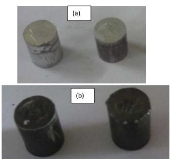
Fig. 4.11: Image of green (a) and sintered (b) body prepared through powder metallurgy process.
