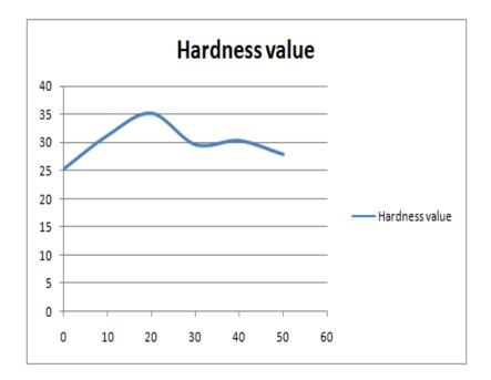
Fig. 4.14: Vickers hardness with respect to the percentage composition of alumina.
