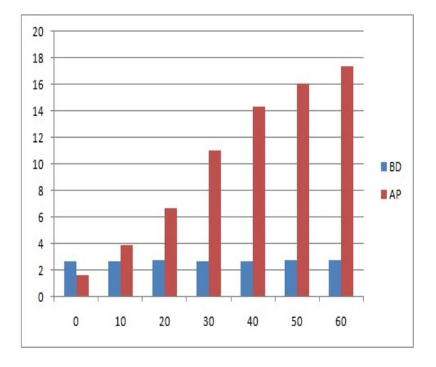
Fig. 4.12: Chart showing the variation of apparent porosity and bulk density of the green body.
