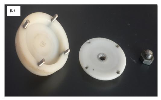
Fig. 3.1: (a) and (b) shows CAD drawing and photograph of the final mould design.
