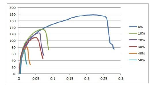
Fig. 4.15: Bending stress versus bending strain of the composite at various compositions.
