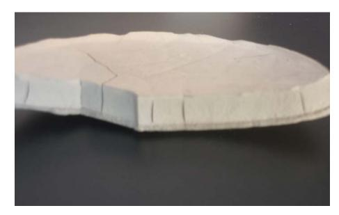
Fig. 4.5 Composite made of gelcasting in conventional way.
