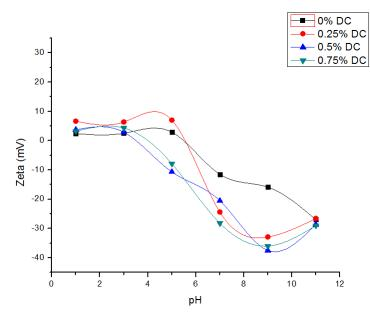
Fig.4.1: Zeta potential versus pH curves at different concentrations of deflocculating agent for preparation of aluminium slurry for gel casting.
