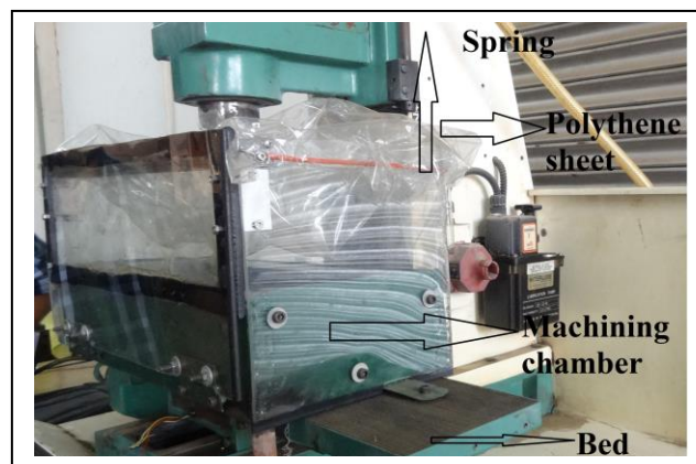
Fig. 7-making air tight chamber by using polythene sheet
