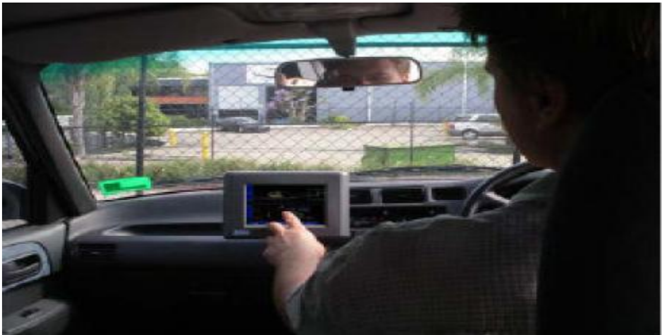
FIG: 5: Foreman's vehicle system equipped with wireless LAN to duplicate Shovel operators view.
